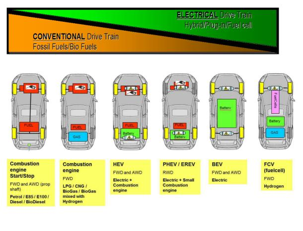
The step from HEVs to PHEVs is a technological challenge. HEV batteries are designed for maximum power where the electrical drive works as a power booster in the vehicle. PHEV require a larger and more expensive battery which needs to be able to store electrical energy instead of power is a less mature technology. Future regulations regarding safe handling of new batteries and fuels in the production line are unclear.
