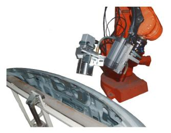
Figure 3. Automatic inspektion cell based on thermography.
