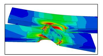
Figure 2 Simulation of tensile test of spot weld joint on boron steel.
