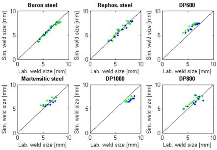
Figure 1 Comparison between measured and predicted spot weld size at first weld location (green) and at second (blue).
