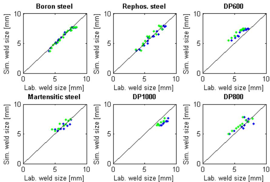
**Figure 1 Comparison between measured and predicted spot weld size at first weld location (green) and at second (blue).**
