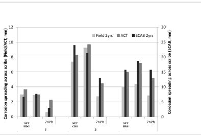
Figure 18. Correlation between ACT results from 2010 and field test with exposure from October 2010 till May 2012.
