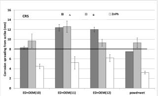
Fig 12. Summarized ACT results from CRS coated with the same paint system (electrocoat + 3 layer paint) for three consecutive evaluations as well as one paint system with powder primer and wet top coat. Requirement for passing is  $\leq 8$ mm corrosion spreading.
