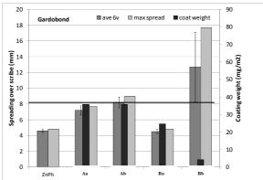
Figure 14 . Results from ACT test on Gardobond C (DC04), reference panels sold by Chemetall.
