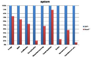
Figure 19. Comparison between ZnPh and new pretreatment. ZnPh was set to 100% for all parameters that were evaluated. GWP= global warming potential.
