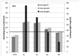
Figure 15. Results from ACT on VCCs cold rolled steel sheet material.
