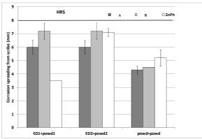
Fig 13. Summarized ACT results from HRS coated with three different paint systems. Two systems with different electrocoat and different powder to coat, as well as a system with powder primer and powder top coat. Requirement for passing is  $\leq 8$  mm corrosion spreading.
