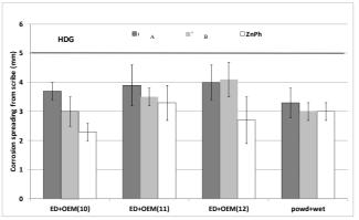
Fig 11. Summarized ACT results from HDG coated with the same paint system (electrocoat + 3 layer paint) for three consecutive evaluations as well as one paint system with powder primer and wet top coat. Requirement for passing is  $\leq$  5mm corrosion spreading.
