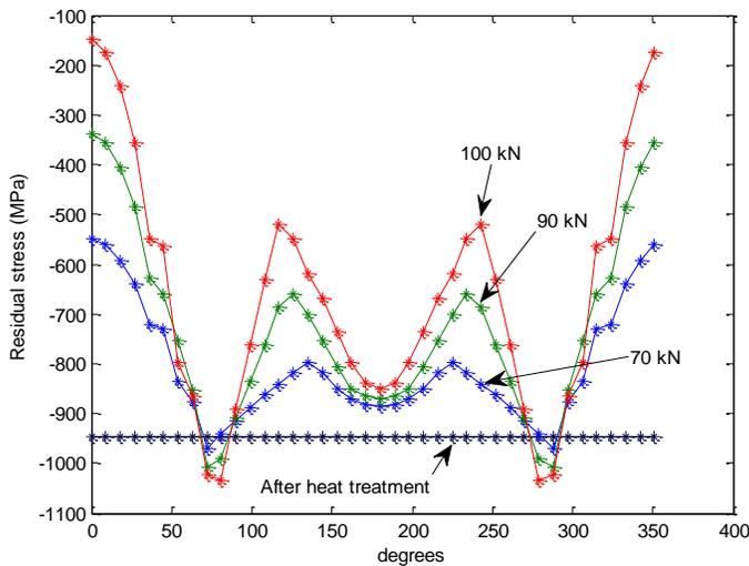
Figure 8 The effect of different straightening force on residual stresses.
