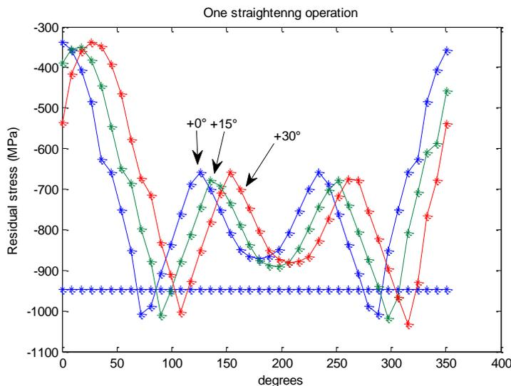
Figure 10 The effect of different direction of straightening force on residual stresses after 1<sup>st</sup> stroke.
