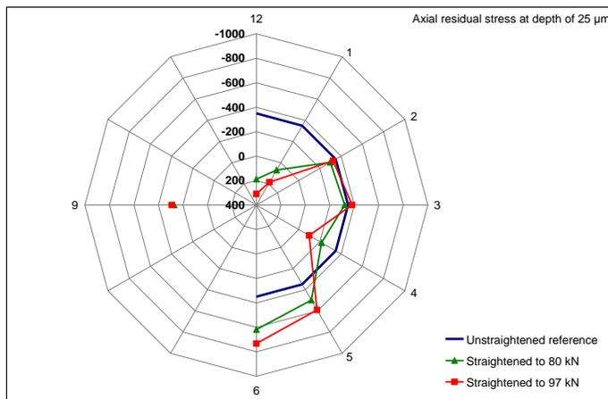
*Figure 7 Polar plot of axial residual stress at 25 µm*
