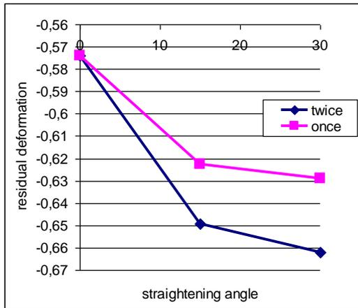
Figure 11 The effect of different direction of straightening force on residual deformation after 1<sup>st</sup> and 2<sup>nd</sup> stroke.
