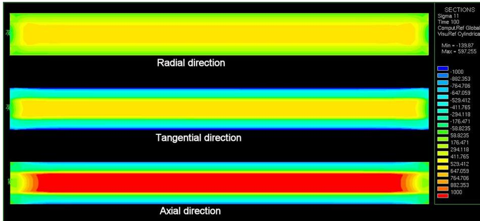
Bild 4 Calculated residual stresses after heating and quenching
