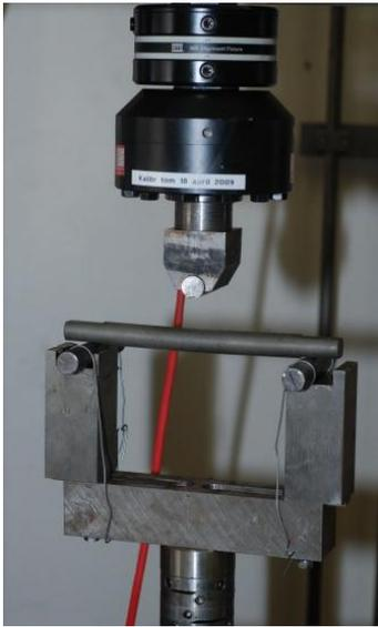
*Figure 1* Experimental setup for fatigue testing
