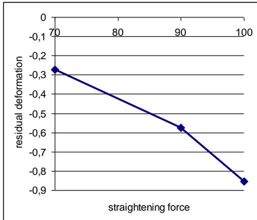
Figure 9 The effect of different straightening force on residual deformation.
