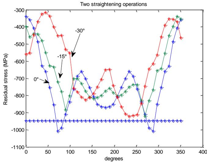
Figure 11 The effect of different direction of straightening force on residual stresses after 2<sup>nd</sup> stroke.
