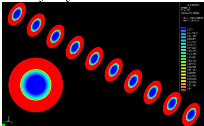
Bild 3 Martensite distribution in the shaft in axial direction. In lower left a magnification of the distribution in the z-x-plane is shown
