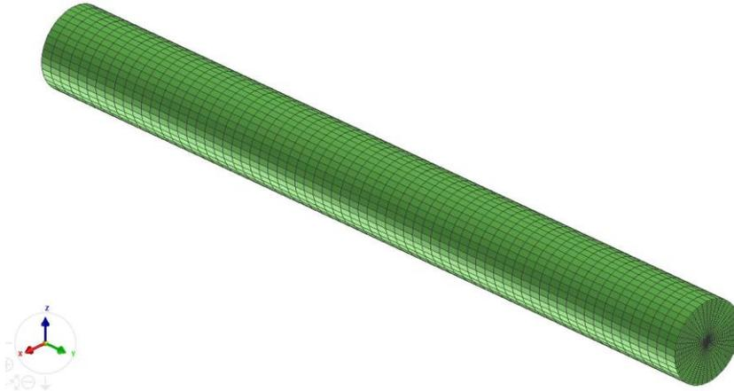
Figure 2 Meshed geometry for the simulated shaft with 67200 element/57871 nodes
