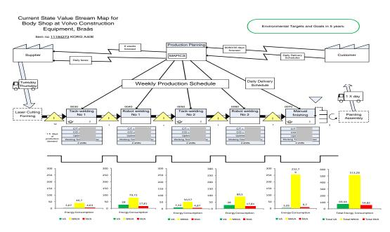
Figure 7. Environmental VSM for the Braås body welding, five stations.
