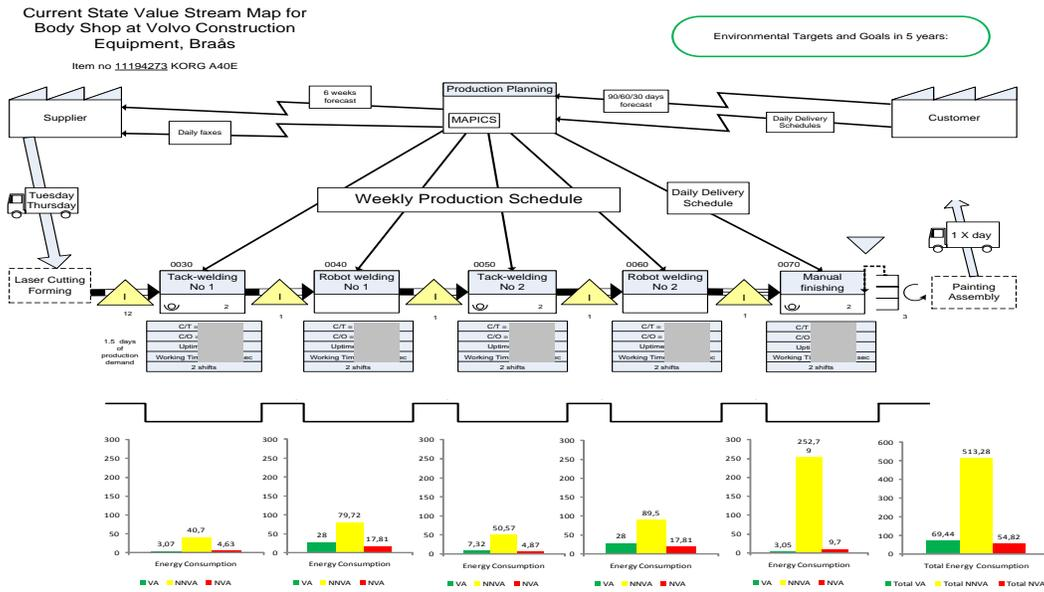
**Figure 7.** Environmental VSM for the Braås body welding, five stations.
