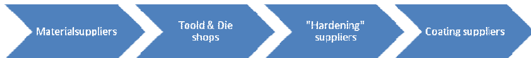
Figure 2. Example of a supply chain that is active in the manufacture of sheet forming tools.
