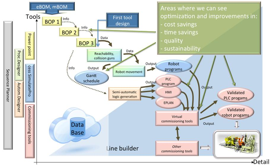
Figure 5 Identified areas where optimization and improvements with in the area of virtual preparation and commissioning can be achieved.
