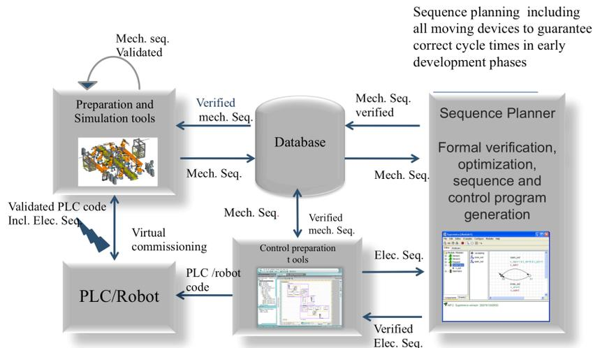
Figure 4 Proposed workflow for preparation of control of a production system
