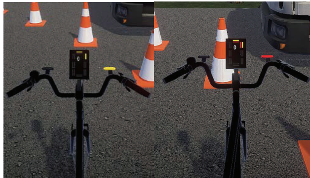
Figure 8. The handlebar in the virtual environment showing the yellow alert (left) and red warning (right).
