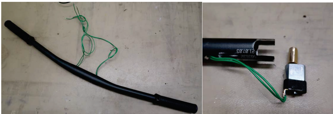
Figure 4 Handlebar integrated with motor on the grip region to produce vibration
