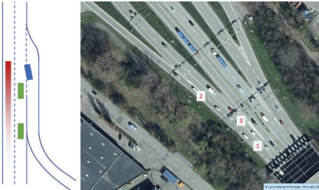
Figure 3. Left: a schematic view of a ramp layout chosen for data collection. Right: An example of a ramp that is deemed unsuitable for data collection. (1) there is an entrance to a tunnel, (2) the acceleration section is not long enough, and its width starts decreasing immediately at the start of merging section, and (3) the solid road marking prevents vehicles in the left lane to change it. Image source: Eniro, © Lantmäteriet/Infotrader i Ronneby AB.
