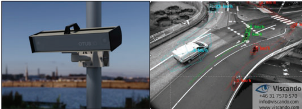
Figure 5. Left: a photo of Viscando OTUS3D sensor installed on a pole. Right: example of tracking of different road users in an urban environment.
