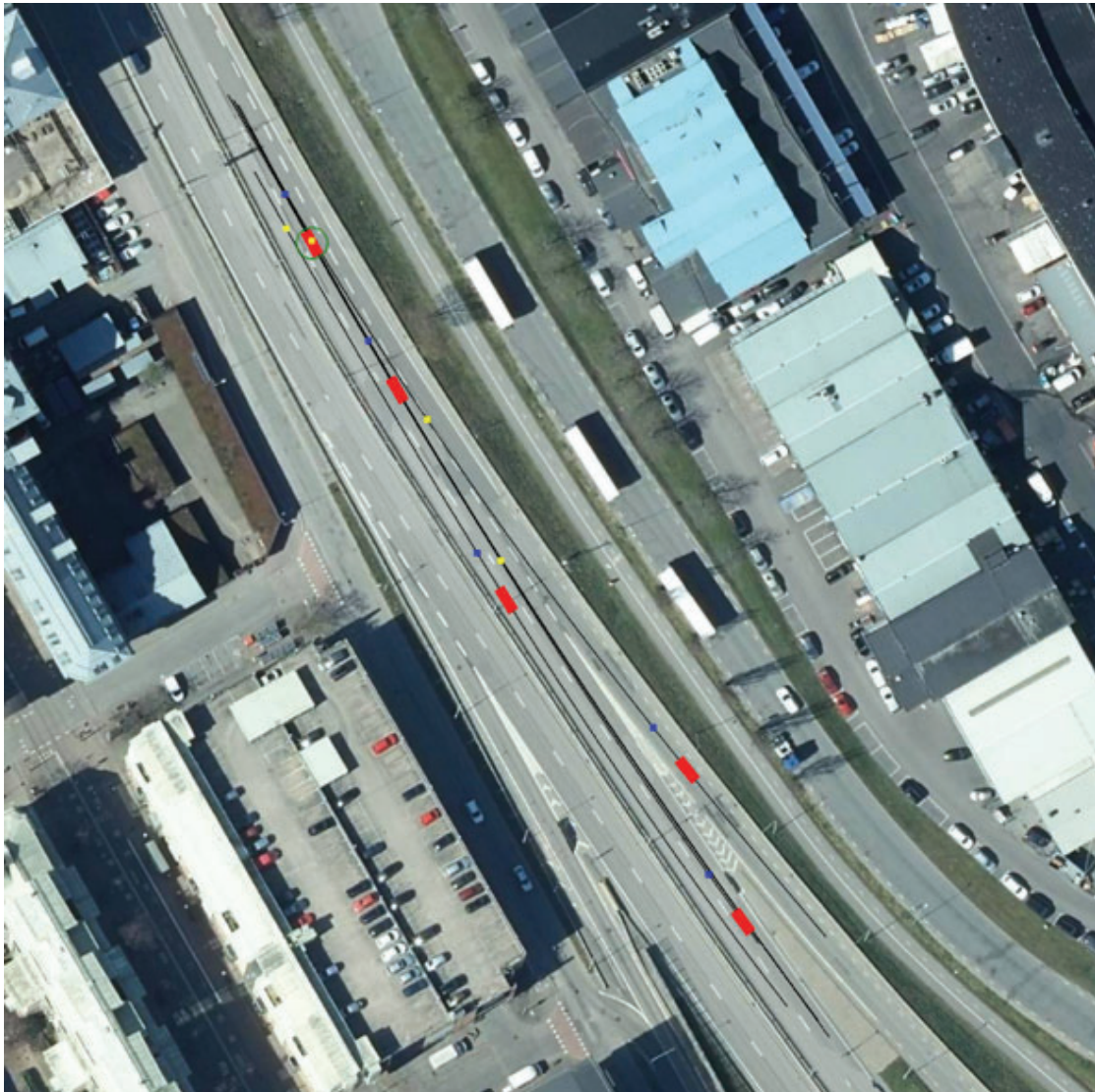
Figure 38. The simulation environment. The red rectangles represent cars, where non-circled cars are replayed directly from data, and the circled car is simulated in closed loop, with a initial state extracted from data. The blue points are the near points, and the yellow the far points. The black lines are the mean path for the three desired paths (left lane, right lane, on-ramp).
