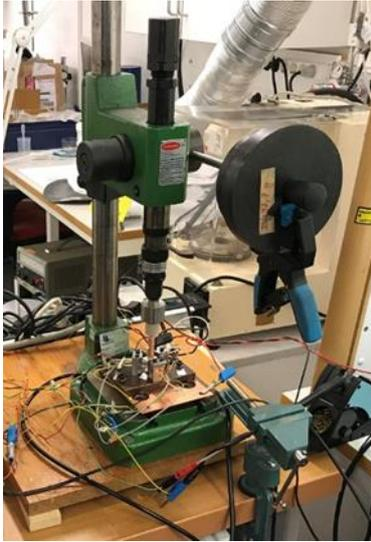
*Figure 2. A measuring fixture was made to be able to measure the resistivity of rods*
