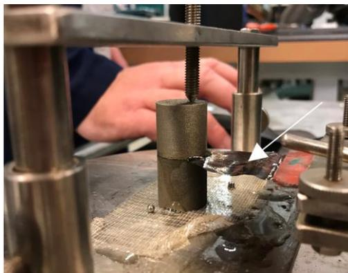
Figure 4. Sample holder with two rods and the sensor clamped in between (the arrow points at the sensor).
