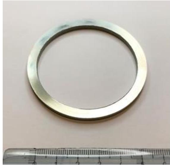
*Figure 1. A ring cut from the "tower" in **Error! Reference source not found.** by using a precision cutting machine*
