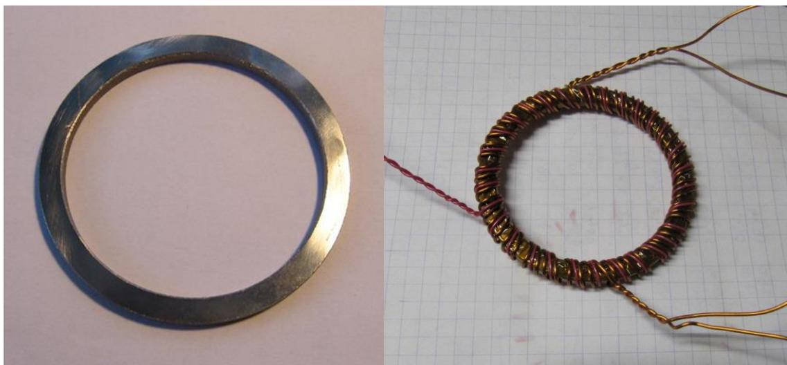
Figure 7. Typical Sample to the left and sample with windings to the right.
