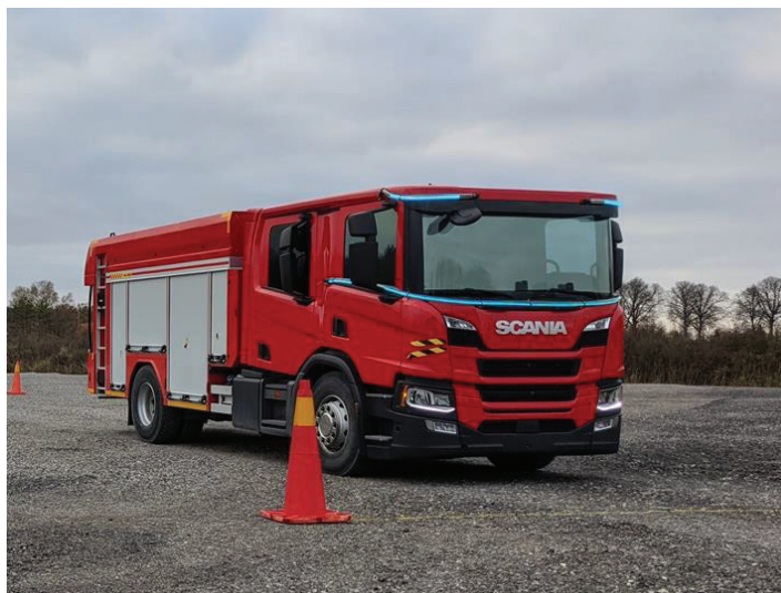
Figure 4 The Wizard of Oz truck with eHMI prototypes on test track in one of our studies with tinted windows and windshield.
