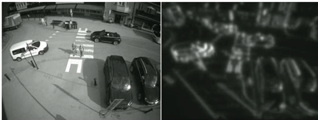
Figure 12: A snapshot of video anonymized using 3D-based anonymization technique described in section 6.6.2. Left image shows original frame, right image the anonymized one.
