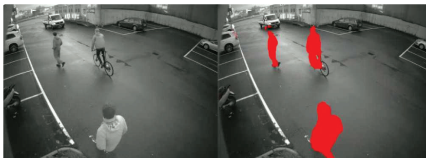
Figure 9: Screenshot of a single frame from a surveillance video provided by Viscando. To the left, the original frame and to the right the automatic segmentation of human bodies in real-time.
