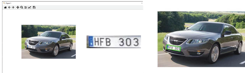
Figure 29: Detected LP from the original image using WPOD algorithm.
