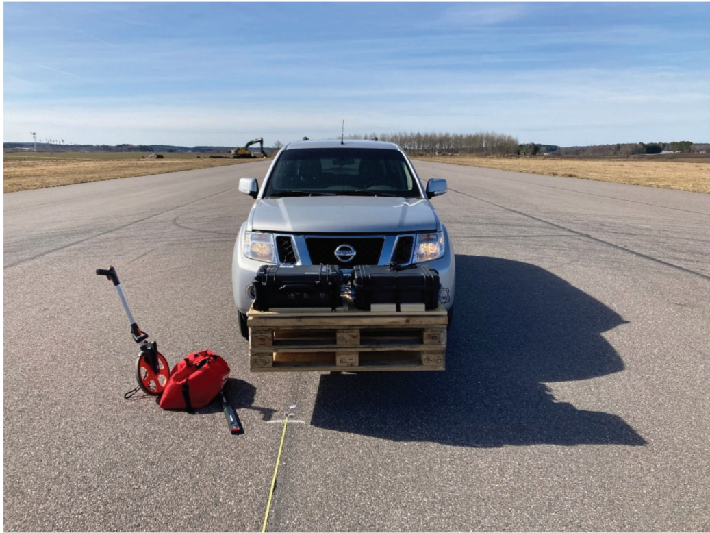
Figure 1 D-Radar ego vehicle setup. The box on the left-hand side containing the radar antennas and the right-hand side containing the digital system.
