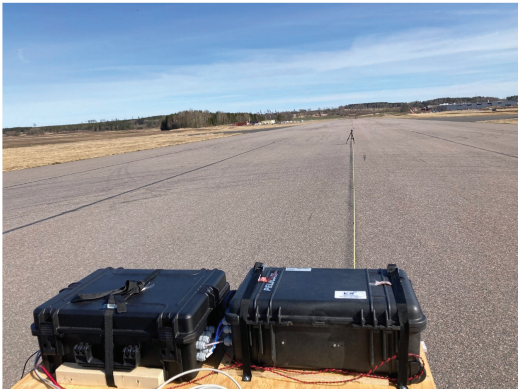
Figure 2 Target corner reflector in boresight of the radar. measuring tape on the ground to measure the distance to the target.
