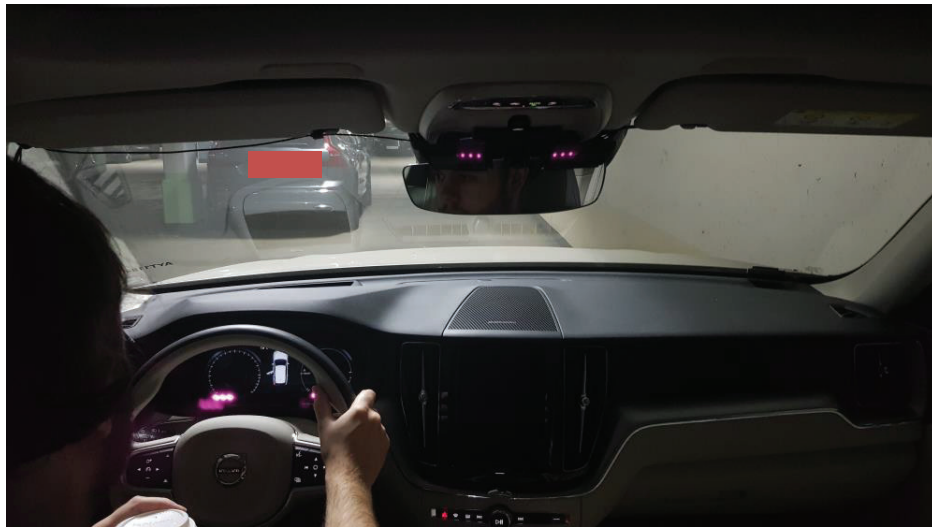
Figure 4. Smart Eye DMS and CMS installation in the data collection vehicle.
