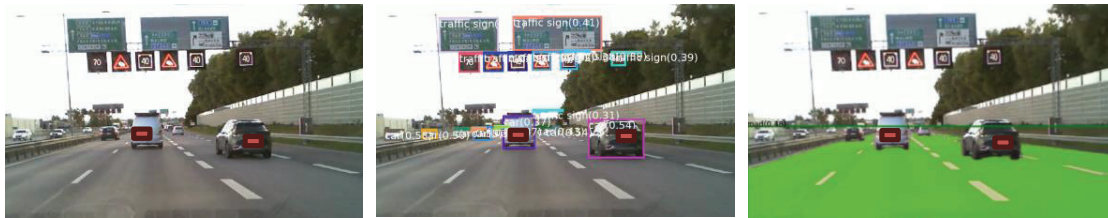
Figure 11. From left to right: Original observation, object detection, drivable road segmentation.
