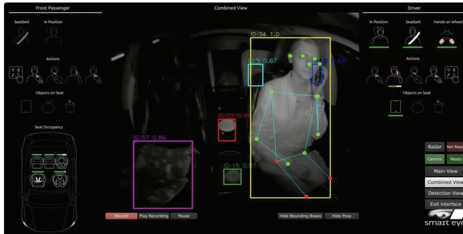
Figure 6. Example of Smart Eye CMS image capture and signals.
