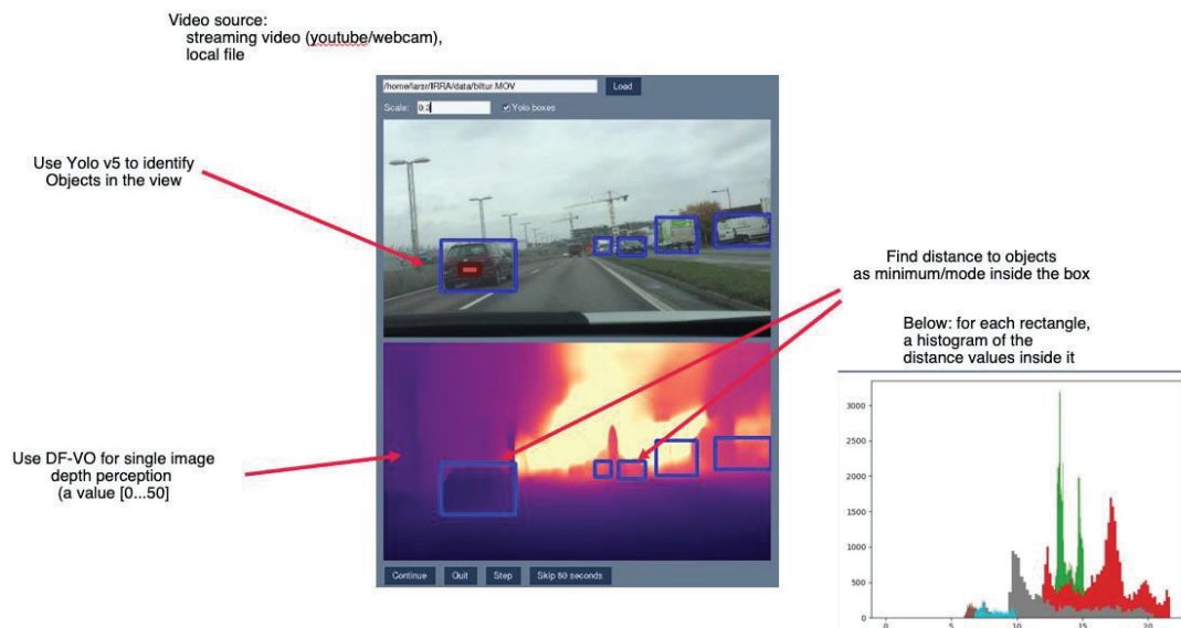
Figure 8. A Vision-to-Distance pre-trained neural network for determining the distances to objects. The histogram to the right shows the distributions of per-pixel distances in the image's bounding boxes as detected by the model (colour coded for the five bounding boxes). The histogram lets us determine the distance of the nearest object to be around 6-7 meters.
