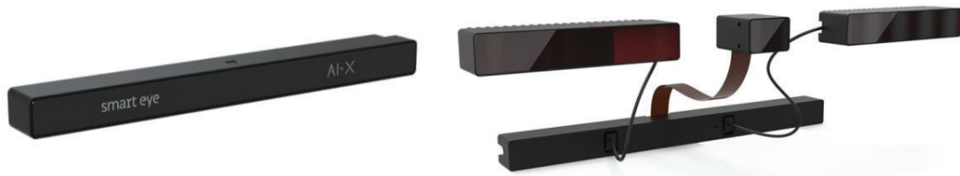
Figure 3. (a) Smart Eye DMS system to the left and (b) prototype CMS system to the right.
