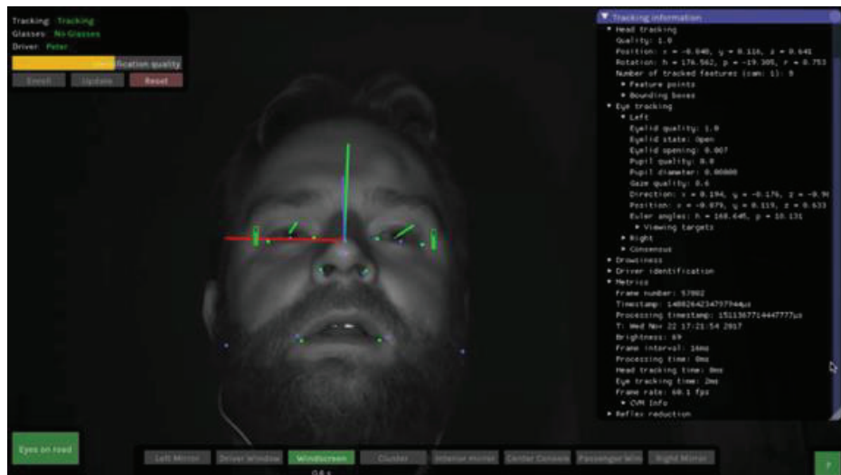
Figure 5. Example of Smart Eye DMS image capture and signals.
