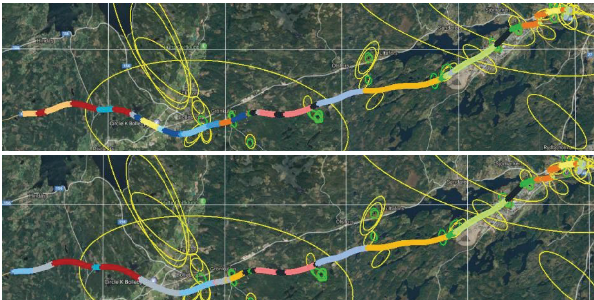
Figure 5.2.2-2. Handover testing for an automotive telematics unit (upper part of figure) and a reference device (lower part of the figure). The different colors indicate connection to different cells. The parameters for each device were logged simultaneously using the same MNO. As can be seen, there are some differences in cell allocations.
