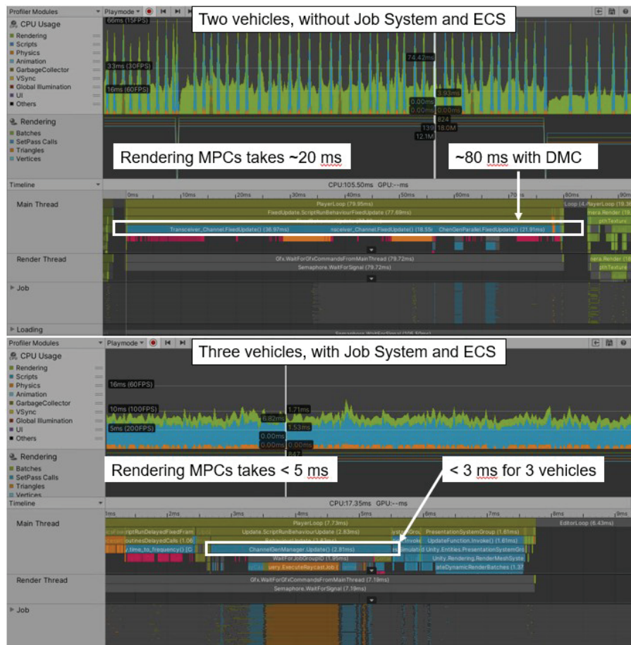
Figure 5.2.1-21. Unity3D Profiler shows the channel modeling execution time. On the top, the performance of channel calculation for two vehicles without the Job System and ECS. On the bottom, the performance of three channel links calculation for three vehicles with the Job System and ECS.
