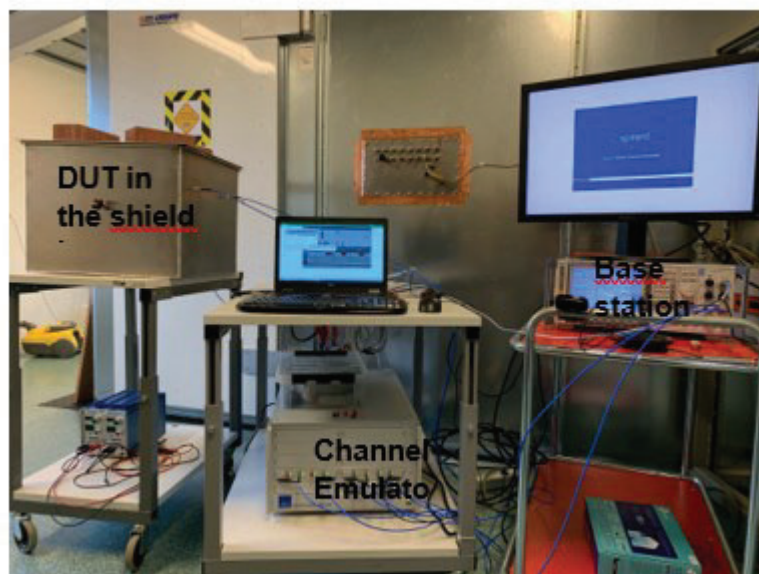
Figure 5.2.2-10. Block diagram of the VDT set-up (top) and picture of the test set-up of VDT inside lab with wireless cable OTA approach (bottom).
