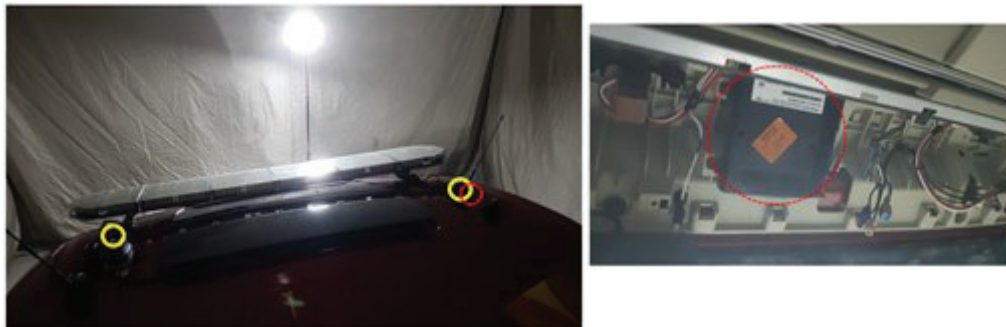
Figure 5.2.3.4-21. Antenna position combinations repeated. On top of cabin (left), in overhead compartment (right).
