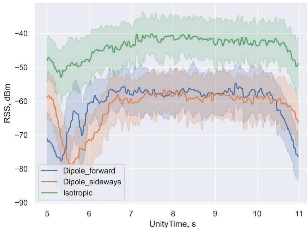
Figure 5.2.1-23. LoS channel for 3 reference antennas.
