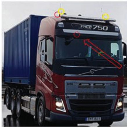
Figure 5.2.3.4-20. Antenna position combinations from outside. Dashed red + red circle: external antenna in combination of antenna in overhead compartment inside cabin. Yellow circles: two externally mounted antennas on top of cabin.
