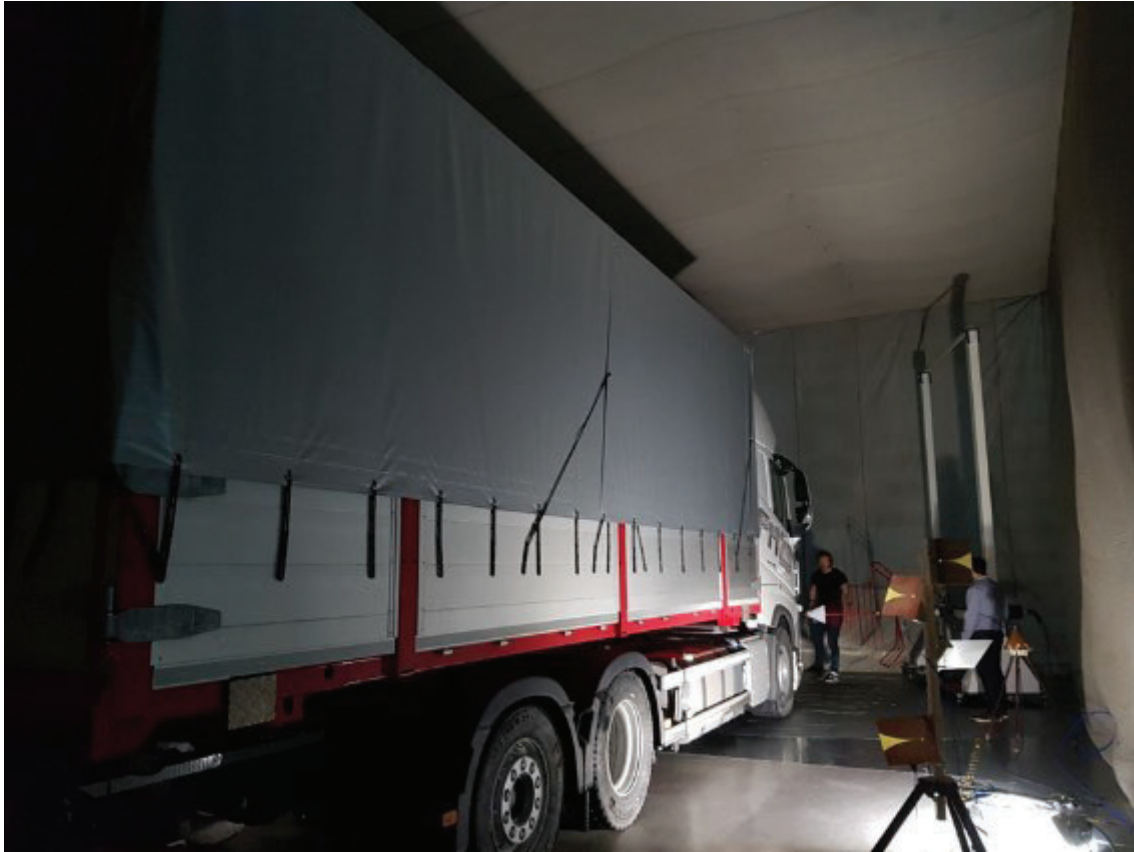
Figure 5.2.3.4-4. Picture of RC tent from inside with a DUT truck.
