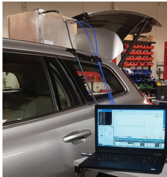
Figure 5.2.3.2-5. Rooftop shielded box (also named car box).
