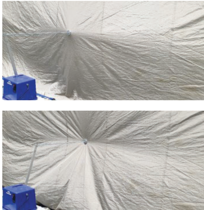
Figure 5.2.3.4-6. Two pictures of a continuous mode stirrer. The movement of the motor creates waves in the textile walls (and roof to some extent). Two motors are built, and they are placed on opposing long sides of the RC tent before test.
