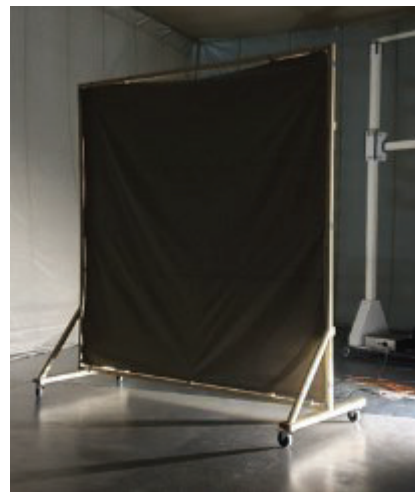
Figure 5.2.3.4-5. Sand filled water hose to secure tent-to-ground connection (left), and a movable shielding wall (right) for reduction of the direct coupling.
