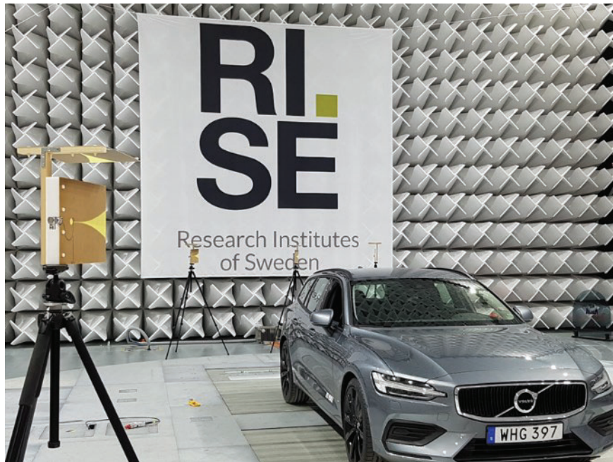
Figure 5.2.3.2-6. Example of test setup in AC with a VUT. Four downlinks and one uplink.
