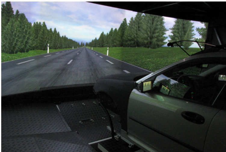
Figure 37 The SAAB 9-3 cabin inside the simulator dome.
