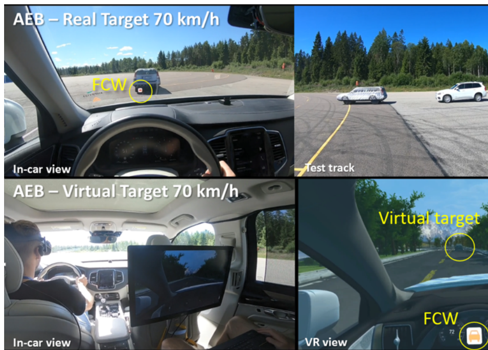
Figure 48. Comparison of real (top) and virtual (bottom) testing of the same automatic emergency braking (AEB) scenario. The virtual target correctly triggers the forward collision warning (FCW) and then activates AEB.
