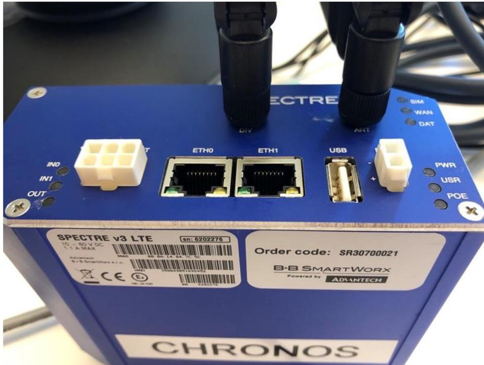
Figure 72 Picture of the Spectre v3 LTE modem used for SUPL/LPP integration. The application developed is run on this device, which in turn is connected to the private 4G network at AstaZero.
