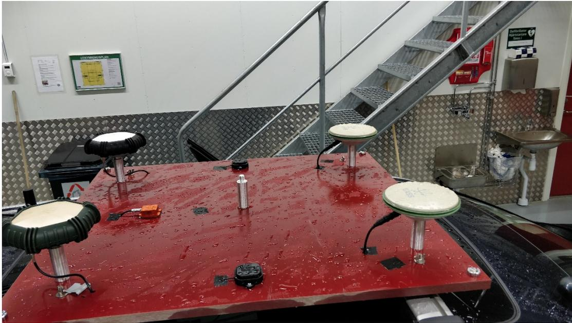
*Figure 78: The current design of the “Leaf” platform, here fitted with 4 geodetic antennas, 2 patch antennas, one IMU and 4 retroreflector mountings. Photo from tests in November 2019.*
