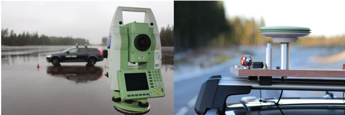
Figure 82: Photos showing the total station heading setup on HSA (left) and the retroreflector used when placed in one of the mountings on the experimental platform during tests at RR (right).
