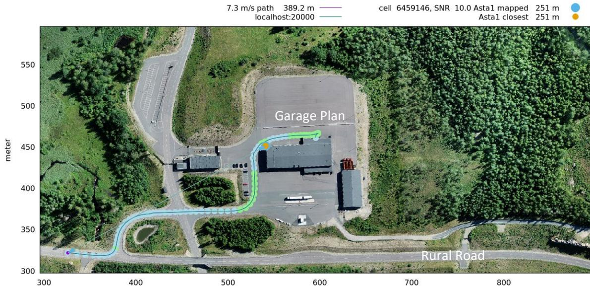
Figure 64 Typical visualization using `check_cells.pl` of tests using an overlay of a local high-resolution aerial photo of AstaZero using `gnuplot`. The scene shows the first few hundred meters of the access road to the Rural Road. Colored dots along the path indicate the cell that was used. The graph indicates the distance to the “cell-chosen” and geometrically “closest” VRS.
