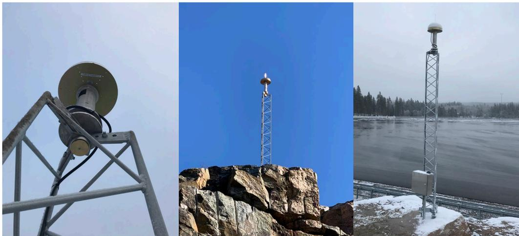
Figure 75: Photos showing the retroreflector mounting below the antennas (left), southern mast which is part of SWEPOS (middle) and the mast next to the high speed area control tower.
