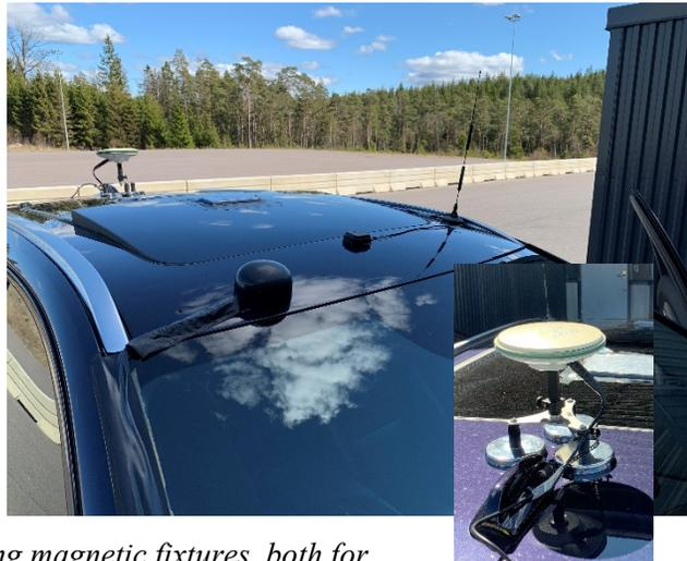
Figure 60 typical ad-hoc antenna setup using magnetic fixtures, both for GNSS antennas and LTE antenna. Power was supplied by the vehicle with backup using a LiFePO4 based battery pack.
