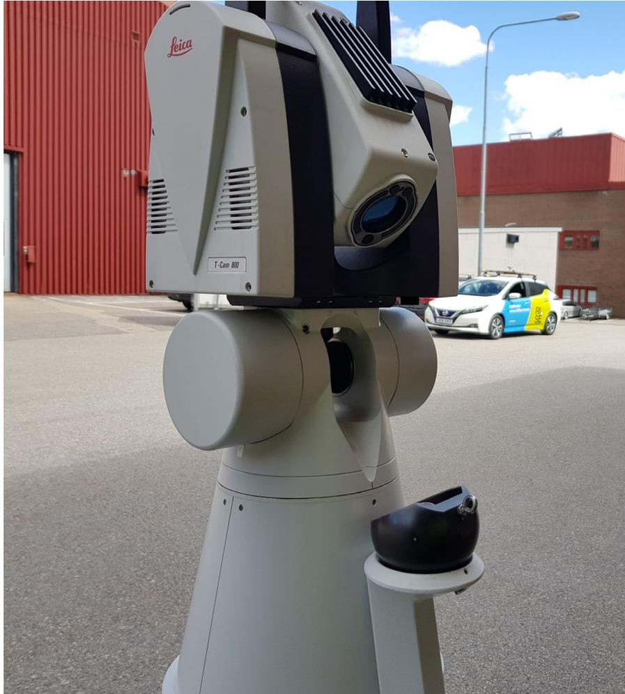
*Figure 79: Laser tracker Leica LTD-800 during outdoor testing and test vehicle fitted with the experimental platform in the background.*
