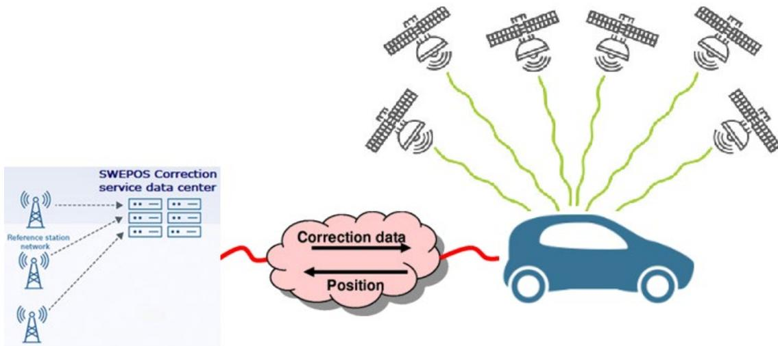
Figure 19 Bi-directional mode used in the traditional SWEPOS technique (VRS).
