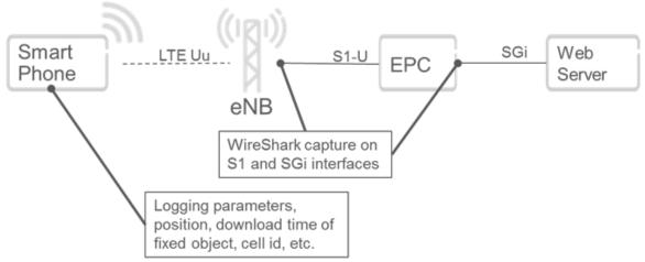
Figure 7.6.3.1: Coverage measurement set-up
