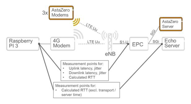
Figure 7.6.3-4: Test set-up for heartbeat measurements
