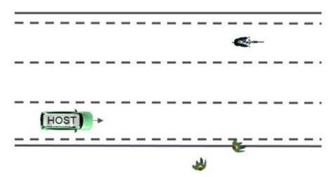
In this case the host is subjected in a city traffic environment where there are multiple Vulnerable Road users (VRUs) that are dynamic in the test space. The VRU's in the space are bi-cyclists, pedestrian, child pedestrian etc. Unlike the usual pedestrian scenarios that are in EUNCAP these pedestrians and bicyclists can move freely in the space and also multi-directional.
