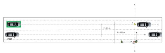
This scenario is similar to Test Scenario 1 with the exception that it is a moving target. The moving target should be a pedestrian which is walking along the road and while the vehicle in front of the host is nearing the pedestrian should start to cross the road.
