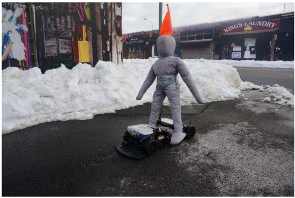
Figure 7.7.3 The RC-car playing the role of a pedestrian.
