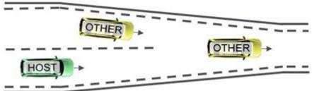
Similar to the above scenario this scenario requires similar decision making capabilities for a HAD car. By varying the position of the target vehicles and by updating the environment in the test system the complexity of the scenario increases.
