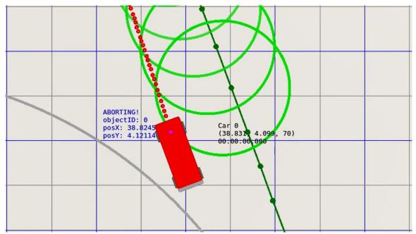
Figure 7.5.2 The visualiser shows the currently considered trajectory point and illustrates the area within which the object must reside (green circle). Alert messages from the supervisor are shown as red points.
