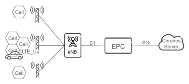
Figure 7.6.2-1: High level 4G architecture at AstaZero
