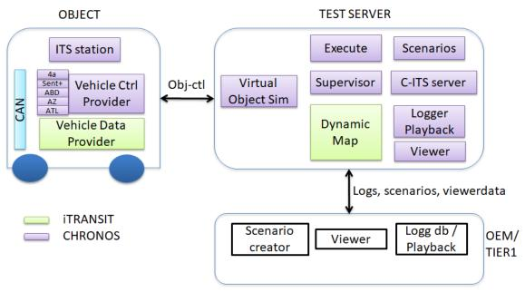
Figure 5 Draft functional architecture, on the system level there are Objects, the cars and targets that are part of a test scenario, and the Test Server. The Test Server controls, monitors and logs test execution, and also interacts with systems on the OEM/TIER1 side.
