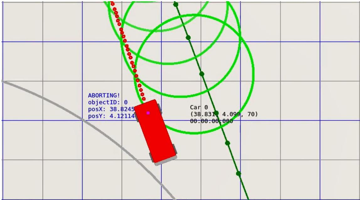
Figure 7.5.2 The visualiser shows the currently considered trajectory point and illustrates the area within which the object must reside (green circle). Alert messages from the supervisor are shown as red points.
