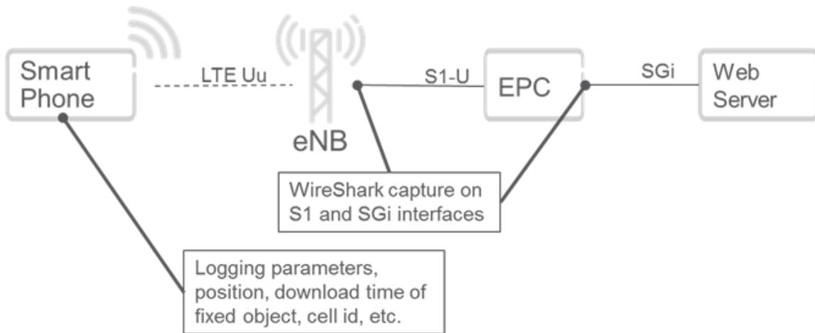
Figure 7.6.3.1: Coverage measurement set-up
