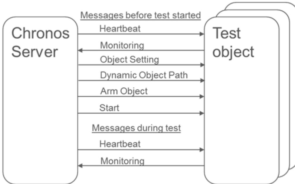
Figure 7.6.2-2: Messages between the Server and Dynamic Object over the cellular network
