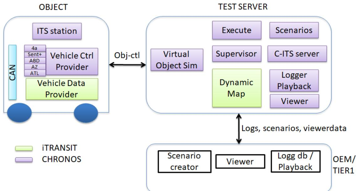
Figure 5 Draft functional architecture, on the system level there are Objects, the cars and targets that are part of a test scenario, and the Test Server. The Test Server controls, monitors and logs test execution, and also interacts with systems on the OEM/TIER1 side.
