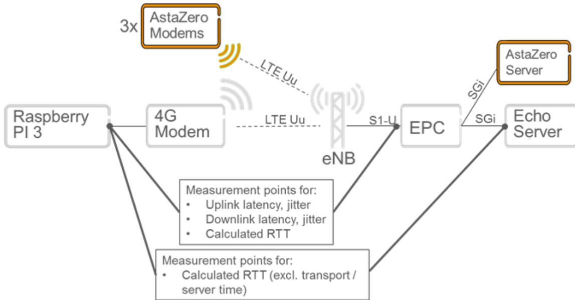
Figure 7.6.3-4: Test set-up for heartbeat measurements
