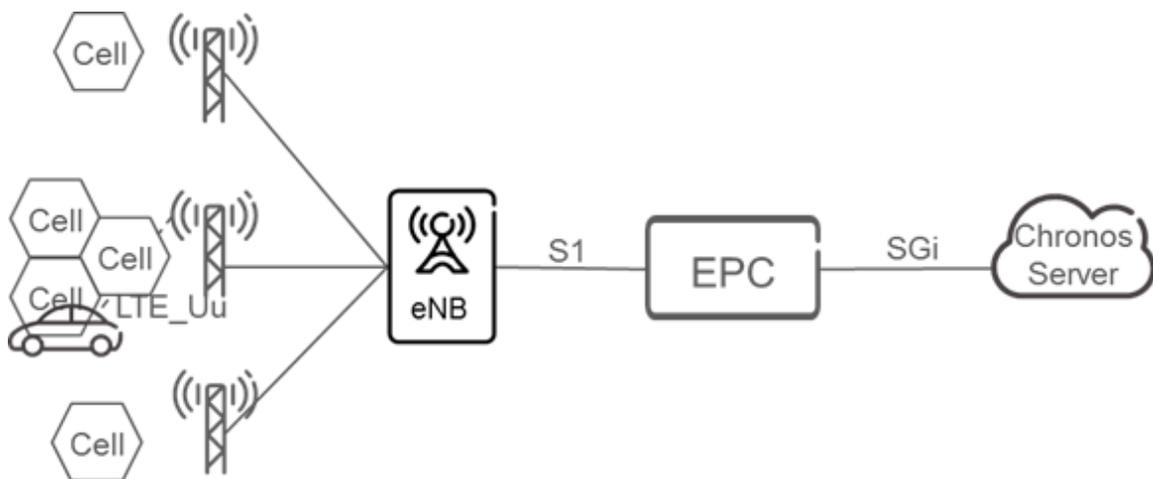
Figure 7.6.2-1: High level 4G architecture at AstaZero
