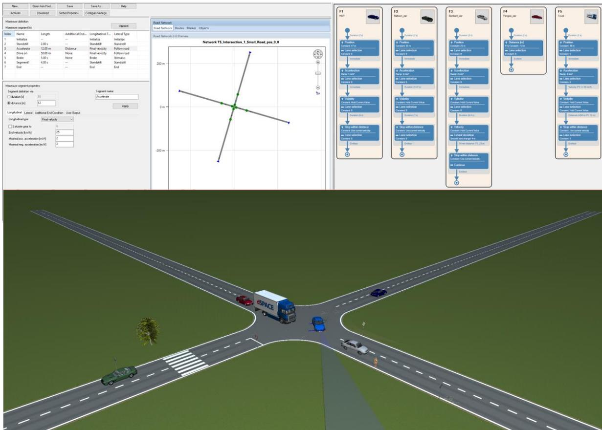
Figure 7.4.3: The GUI for creating a scenario for Drive File-creation together with a simulation of the Final Scenario.
