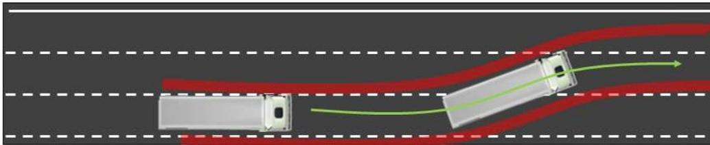
Keeping the distance and follow the trajectory while changing lane. The test case aims on verifying that the time gap (distance) is within the limit values and that the autonomous following trucks are following the trajectory of the lead truck. If the function in the following truck is deviating too much and the red area is entered the driving robot should take over and steer the truck according to the trajectory of the lead truck or make a safe stop of the VUT.
