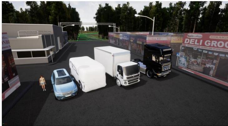
The database of objects now consists of 5 objects but the engine is built to be able to easily extended for other and new scenarios. When connected to the server via UDP the stream of data packages spawn and drive the objects in the running scenario, both virtual and real objects. During a test scenario the user can navigate freely around the test track or follow a selected object. The user can monitor all in data based on the information in the data package.
