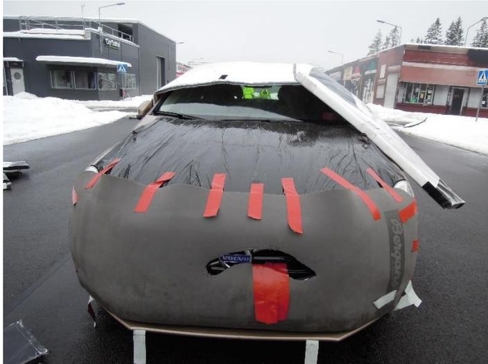
*Figure 39 The Volvo V40 from AstaZero, covered with plastic sheet and foam in the front for impact protection.*
