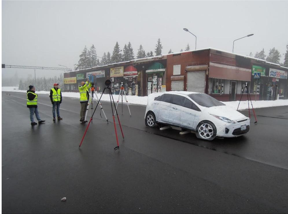
*Figure 48 Geometry scan of the soft car target in the City Area at AstaZero proving ground*
