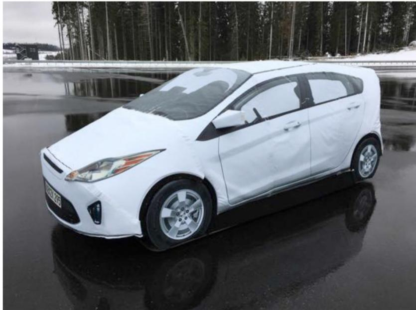
Figure 4 Depicts the latest version of the DRI Softcar 360 target, note the side mirrors, “see through” windows and wheel change compared to Figure 3.
