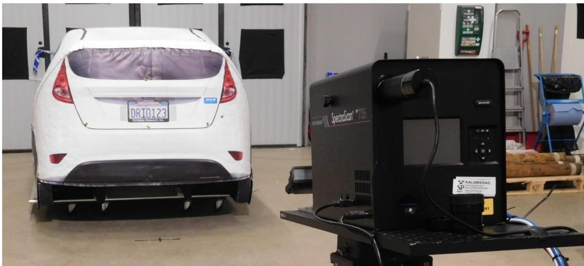
Figure 18. Spectroradiometer and Veoneer camera in the measurement position.
