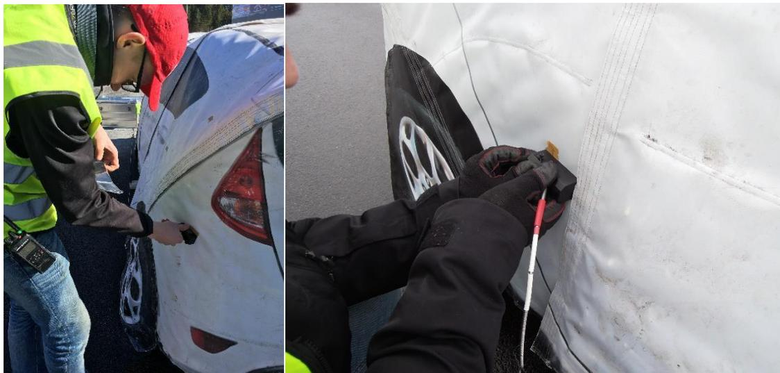
Figure 47 Sampling the optical reflectance in two different points on the soft car target
