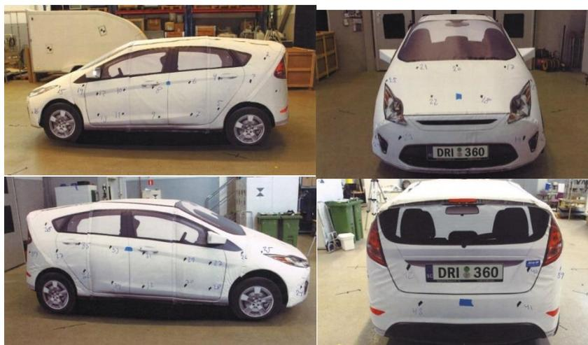
Figure 42 The target with measurement points indicated with pieces of tape.
