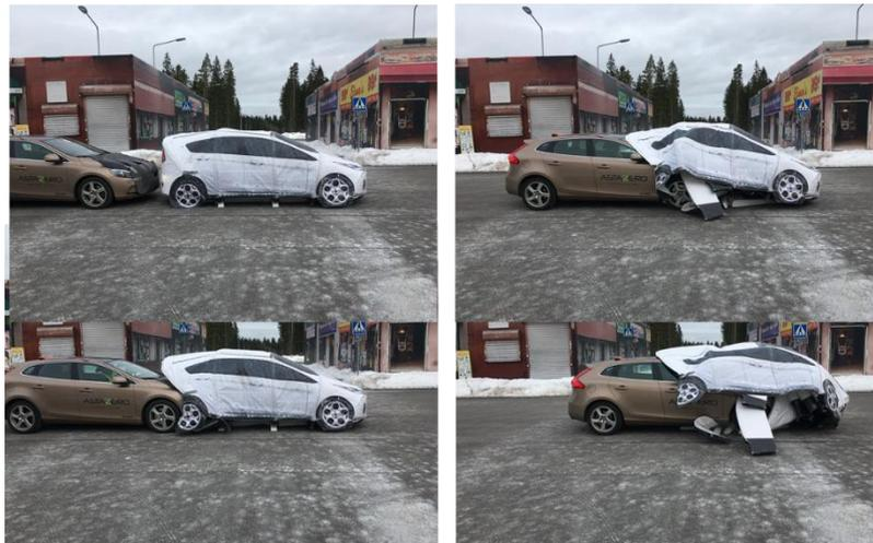
Figure 44 Pictures showing one of the 100 collisions, in this occasion with the Volvo V40
