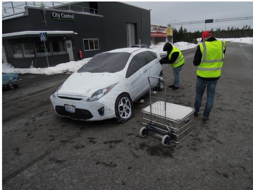
Figure 46 The portable optical reflectance measurement equipment in action
