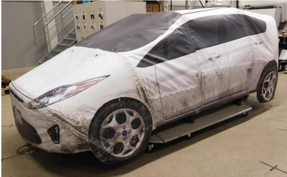
*Figure 16. Soft car target 1 as used in measurements.*
