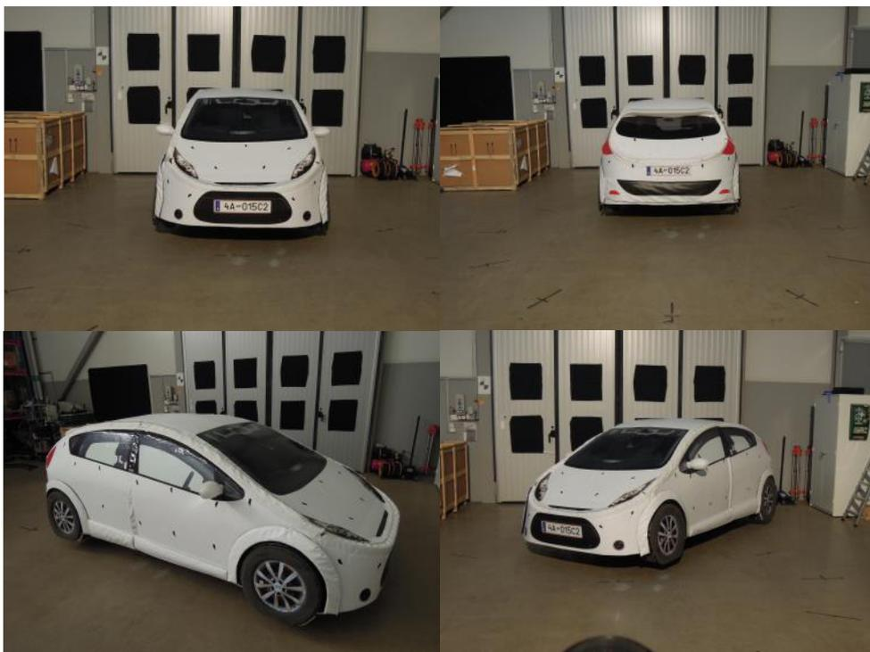
Figure 29 4activeC2 car target set up for measurements at RISE in Borås.
