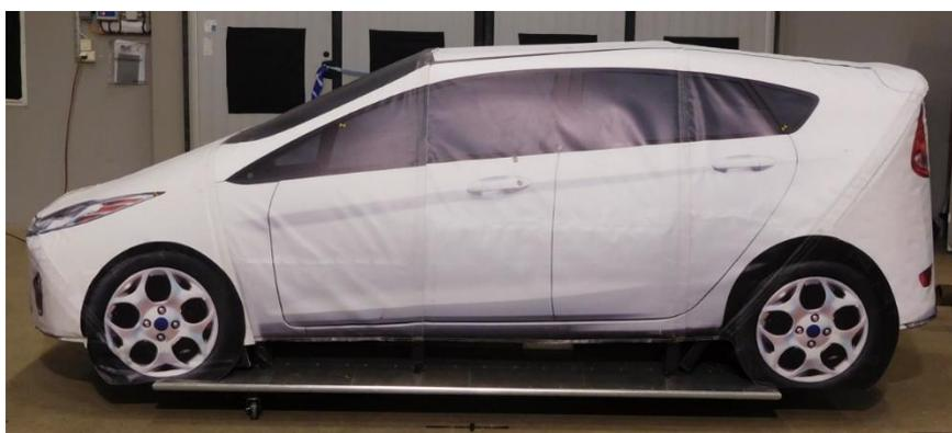
*Figure 36 The Soft Car Target in “mint condition”*
