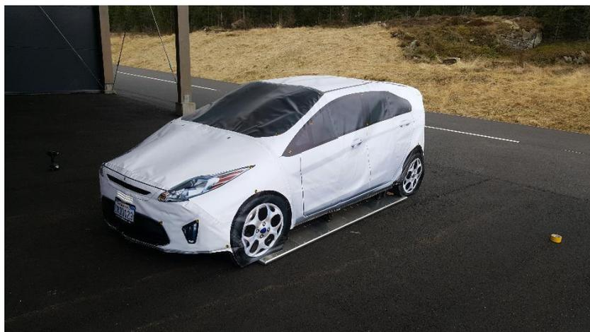
*Figure 8 HSP with the Soft Car 360 mounted.*
