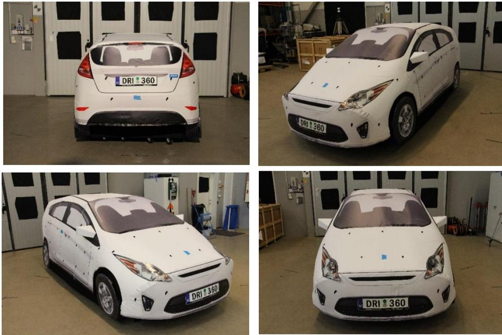
*Figure 30 DRi Soft Car 360 target set up for measurement at RISE in Borås.*
