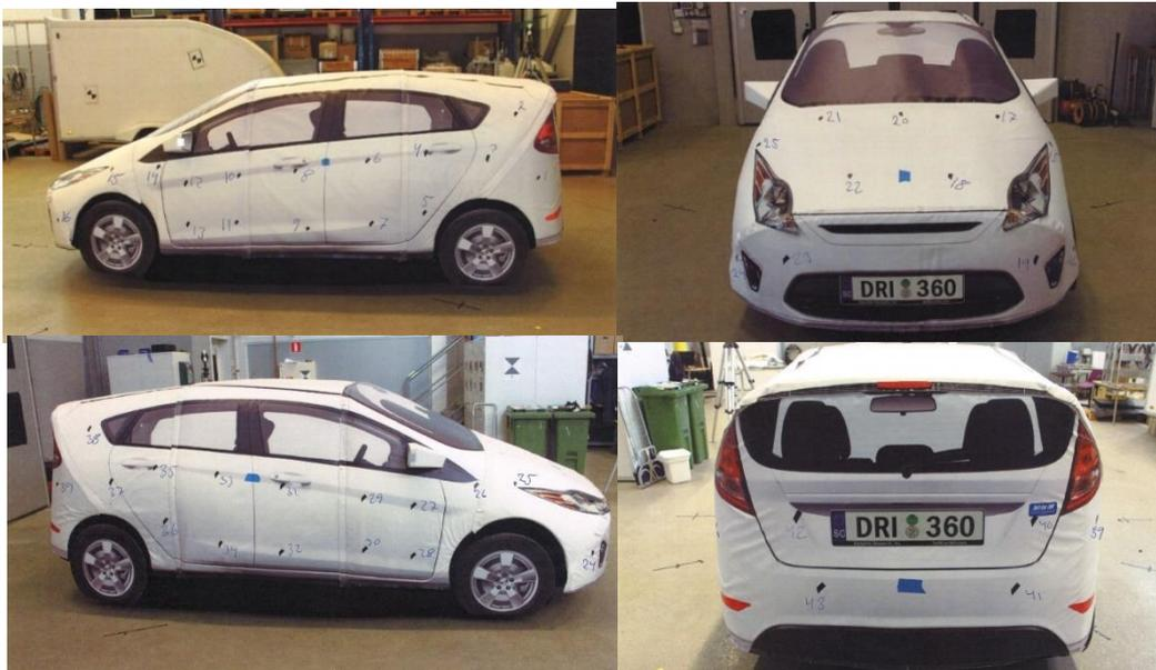
Figure 32 The target with measurement points indicated by pieces of tape.
