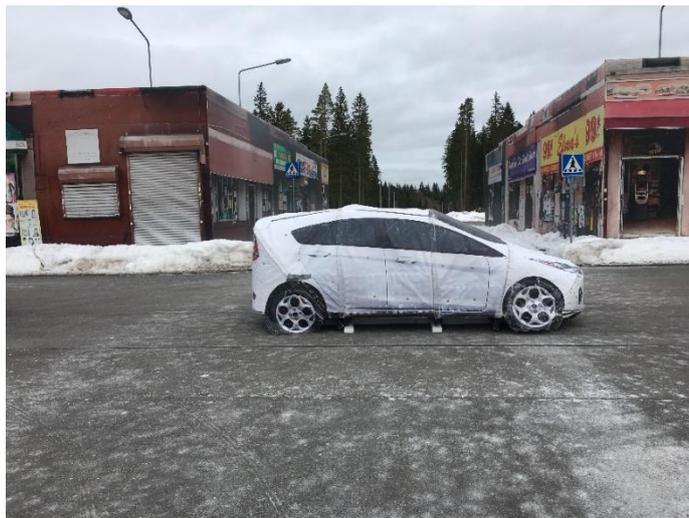
*Figure 35 The Soft Car Target in the City Area of AstaZero proving ground.*
