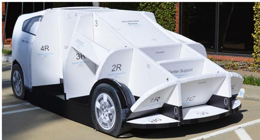
Figure 5 shows the chassis before being covered by the car print sheet [15].
