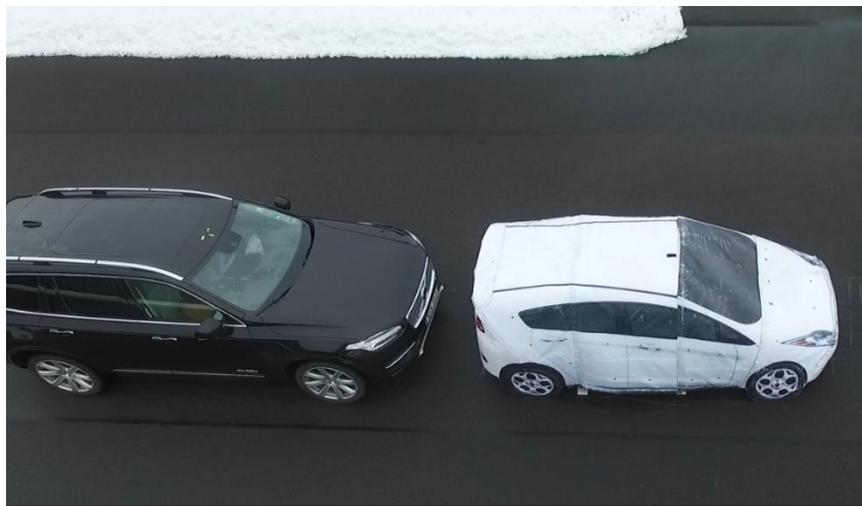
Figure 52 Rear collision scenario in the test track
