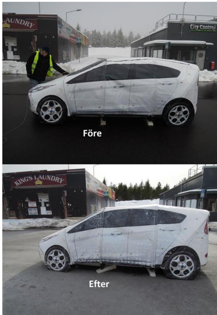
Figure 54 Before (top) and after (bottom) picture of the 3D soft car target
