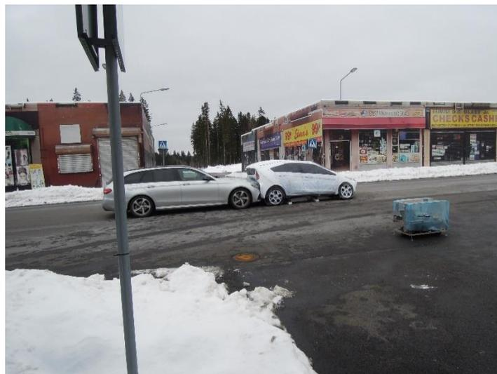
*Figure 38 The Mercedes from Veoneer, prepared with plastic coating in the front for impact protection and equipped with the Veoneer stereo camera system, in order to record raw data.*
