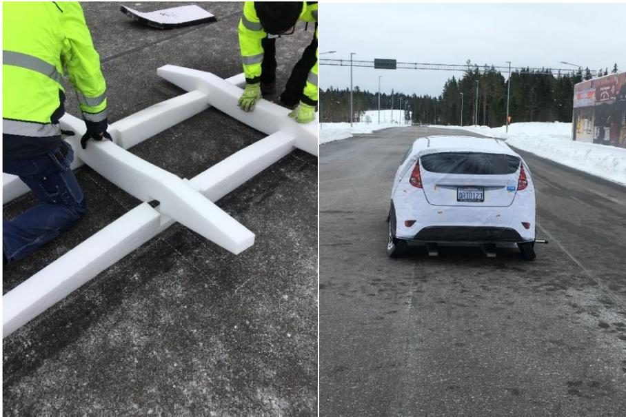
*Figure 37 To the left: The plastic foam support used instead of a real target carrier. To the right: The soft car target assembled on the foam support and ready for collision*
