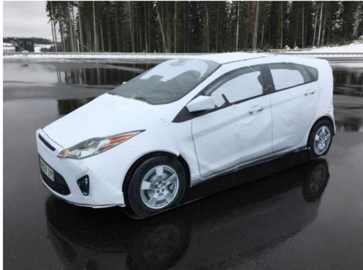
Figure 28 The latest version of the DRI Soft Car 360 target, note the side mirrors, “see through” windows and more realistic wheels.
