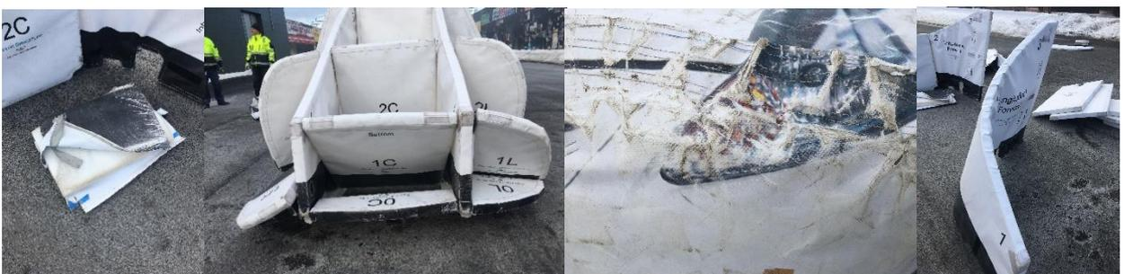
Figure 45 Pictures showing the deterioration of the soft car target
