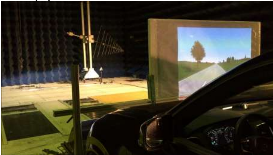
Figure 5: View of the projector screen, and the passive radar target rig during test 1. During test 2, the antenna was angled towards the car and placed much closer.
