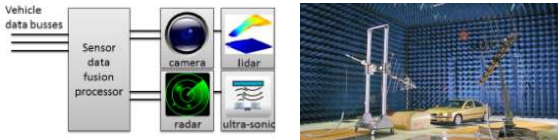
Figure 1. Future vehicle functions will depend also on the robustness of all the multi sensor systems and communication systems of surrounding vehicles and infrastructure (above), illustration of block diagram of sensor data fusion system for vehicle control or warning (below left) and EMC testing facility Faraday at RISE (below right).
