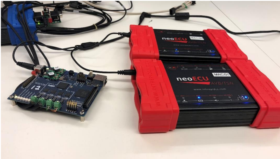
Figure 17. TSN proof of concept with VCC audio use case
