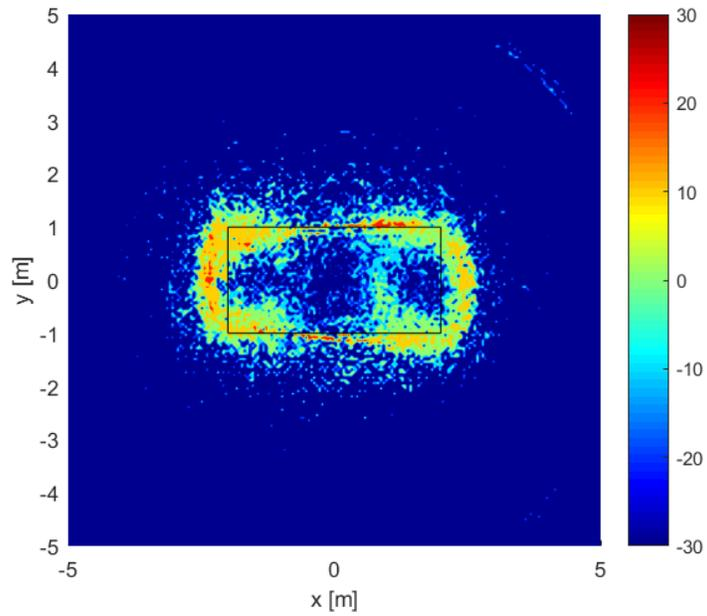
Figure 7. Back projected RCS of a real vehicle.
