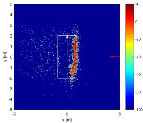
Figure 10. Grid summation RCS image of back projected detections for the surrogate target with the radar located at  $90^\circ \pm 15^\circ$  relative to the target. The color is the calculated RCS in dBm<sup>2</sup>
