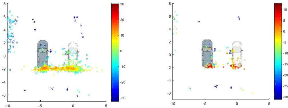
Figure 26. Back projection, onto the targets, of all detections registered during one testcycle with the radar passing between the two targets. The blue/grey target on the left represents a real car and the white target on the right a surrogate. Colorbar shows RCS [dBsm] for individual detections. x- and y-axis show distance [m] from centre. Left: all data. Right: data filtered to only show data from when the radar is closer than 20 m from the target.
