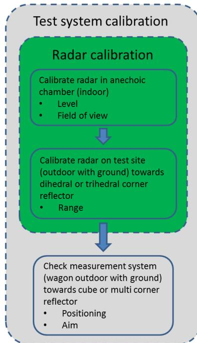
Figure 4. Measurement radar calibration procedure established in the project.
