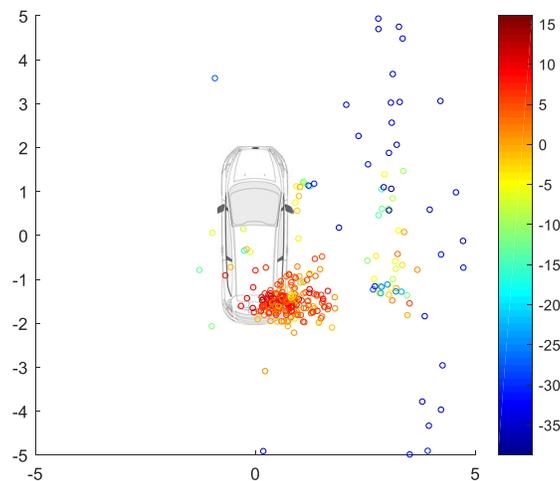
Figure 28. All detections collected during one test with the forward-looking radar mounted on a vehicle passing to the right of the moving target. x- and y-axis shows distance[m] from target center. colormap shows RCS [dBsm] of each detection.
