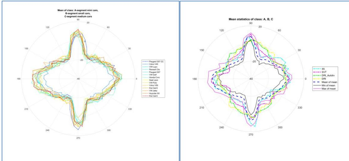
Figure 17. Measured RCS of vehicles from the A-C segment (left). Comparison of the real vehicles RCS to a couple of 3D targets (Right).
