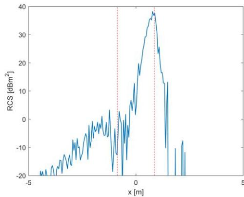
Figure 11. Compared to the figure on the left, RCS spatial profile can easily be completed with limits. This figure shows RCS spatial profile for the surrogate target when the radar is located at  $90^\circ \pm 15^\circ$  relative to the target (positive x is closer to the radar). The dashed red lines mark the approximate physical dimensions of the target.
