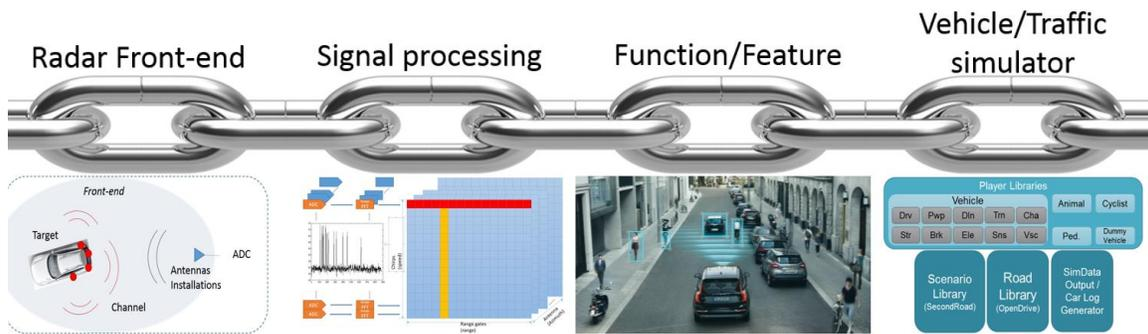
Figure 33. Radar virtual verification tool chain.
