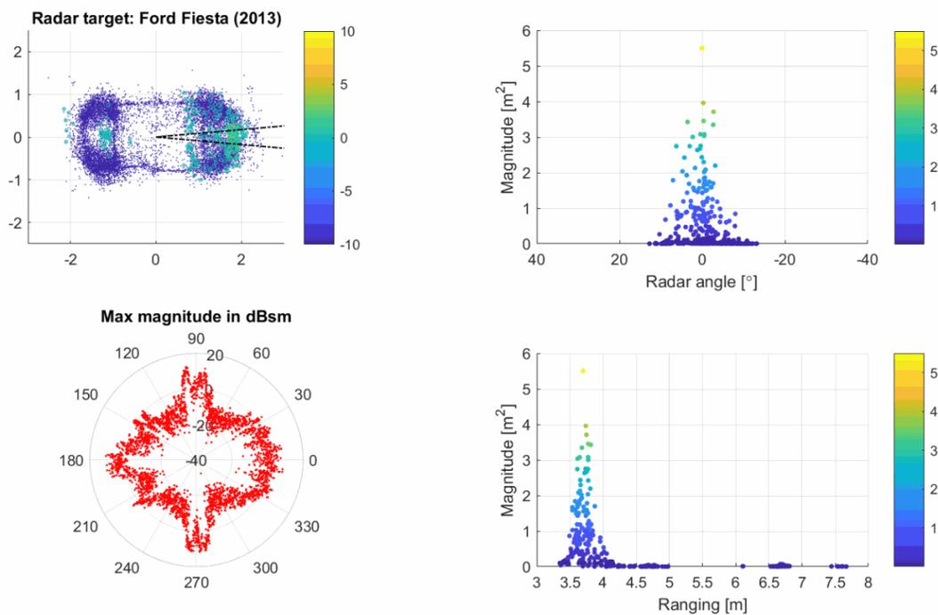
Figure 16. Example of measurement result on a Ford Fiesta. Back projection, RCS as function of angle, RCS spatial distribution as function of radar angle and as function of radar range for a given AoA window.
