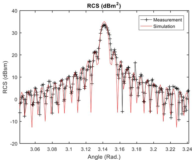
Figure 1. Verification of test method: monostatic RCS over angle of measured and simulated reference cube.
