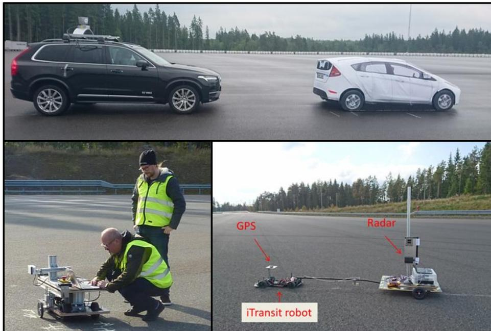
Figure 3. VCC test setup measuring on a DRI surrogate target (upper), the Autoliv RCS measurement chart (lower left), and RISE automotive radar carried by a trolley positioned by the iTransit robot (lower right).
