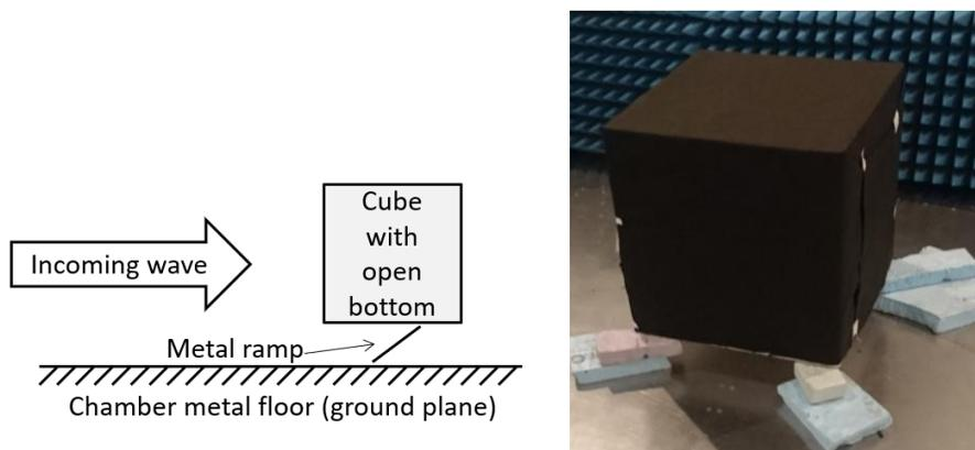
Figure 29. Left: Schematic drawing of test set up. Right: Cube covered in only the RF-absorbing textile inner lining. Layers can be changed or added.
