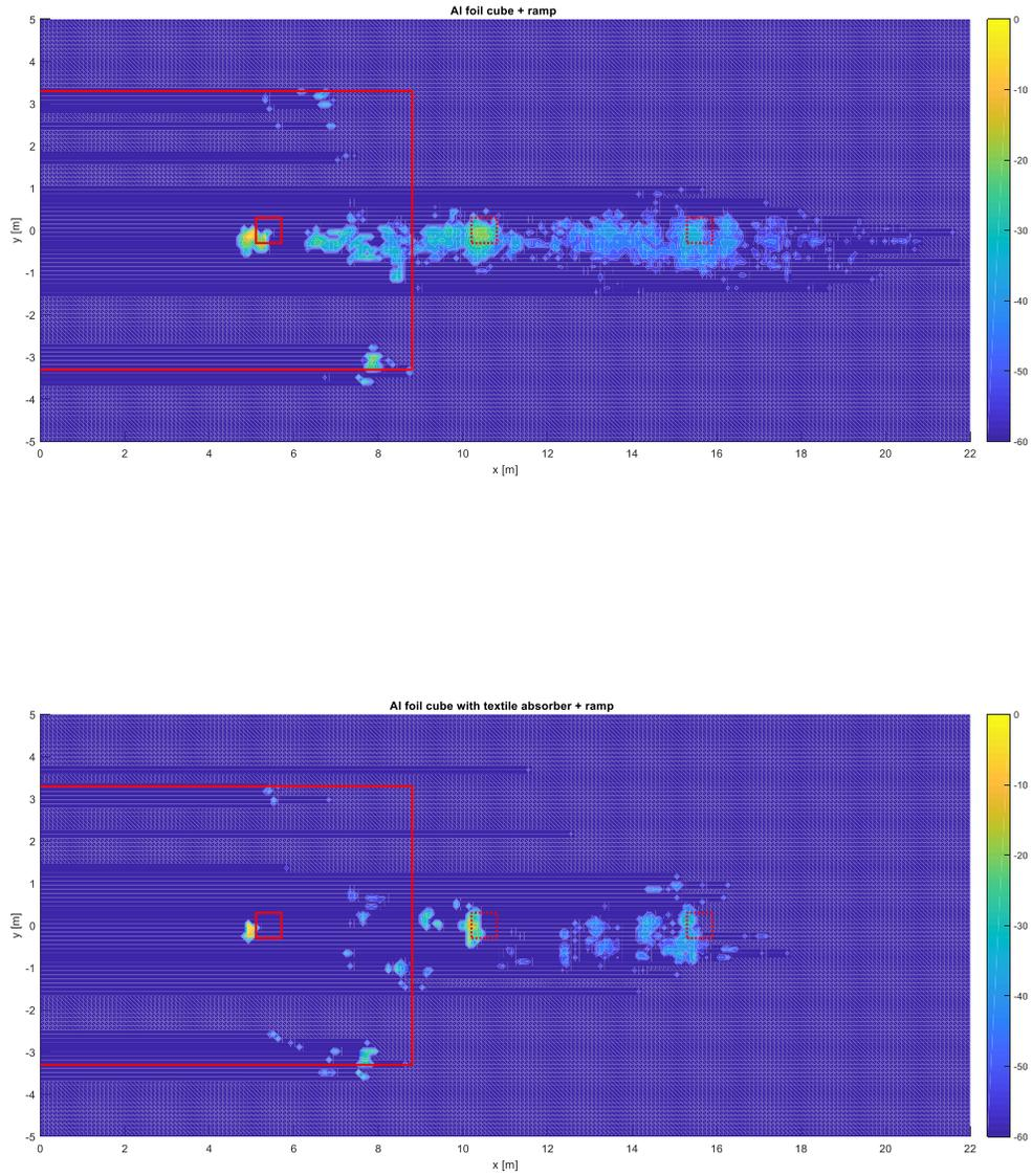
Figure 30. Resulting RCS-probability of the cube when covered in aluminum foil and with a reflecting ramp present underneath (upper), and with an inner lining of RF-absorbing textile (lower). Red squares mark the cube (solid) and the first two predicted "ghost" reflections of it (dotted lines).
