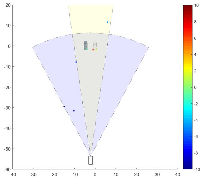
Figure 25. Detections at one time instance of a test scenario with a vehicle carrying the radar (white square) passing between two targets (left car represents a real vehicle and the right a surrogate target). The vehicle carrying the radar has two range modes (medium and far) shown in blue and yellow. Colormap shows RCS [dBsm] for each detection.
