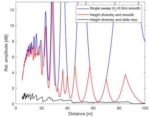
Figure 9. Estimate of the error originating from ground reflection for three approaches to characterize RCS as function of range. Sliding max outperform smoothing method and single height measurement.
