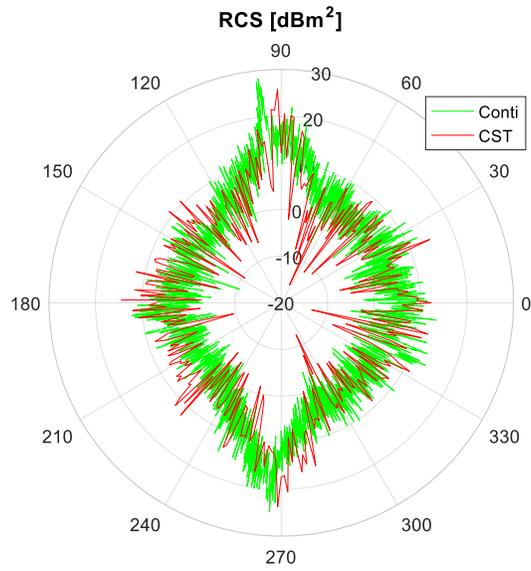
Figure 6. Measured RCS (green) compared with simulation (red).
