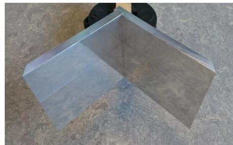
Figure 2. Dihedral corner reflector with reduced reflection into ground.
