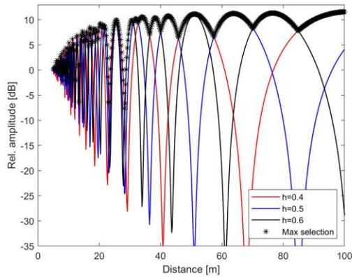
Figure 8. Simulated RCS over range for three different radar heights and height diversity by max selection at each distance.
