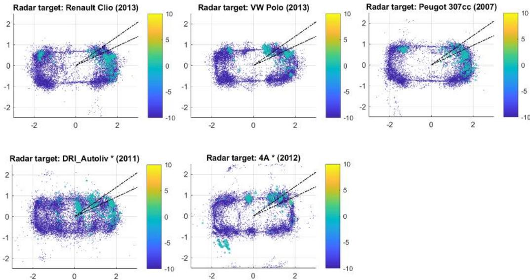
Figure 24. Example of the detection locations and magnitudes of the B class vehicles and some 3D targets at 30°.
