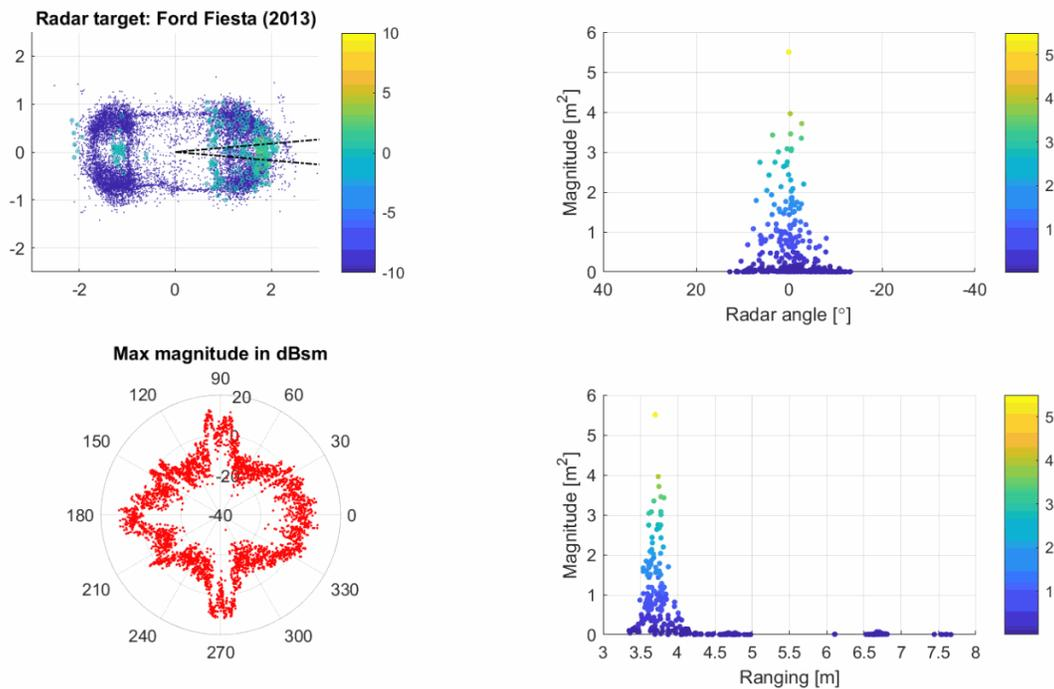
Figure 16. Example of measurement result on a Ford Fiesta. Back projection, RCS as function of angle, RCS spatial distribution as function of radar angle and as function of radar range for a given AoA window.
