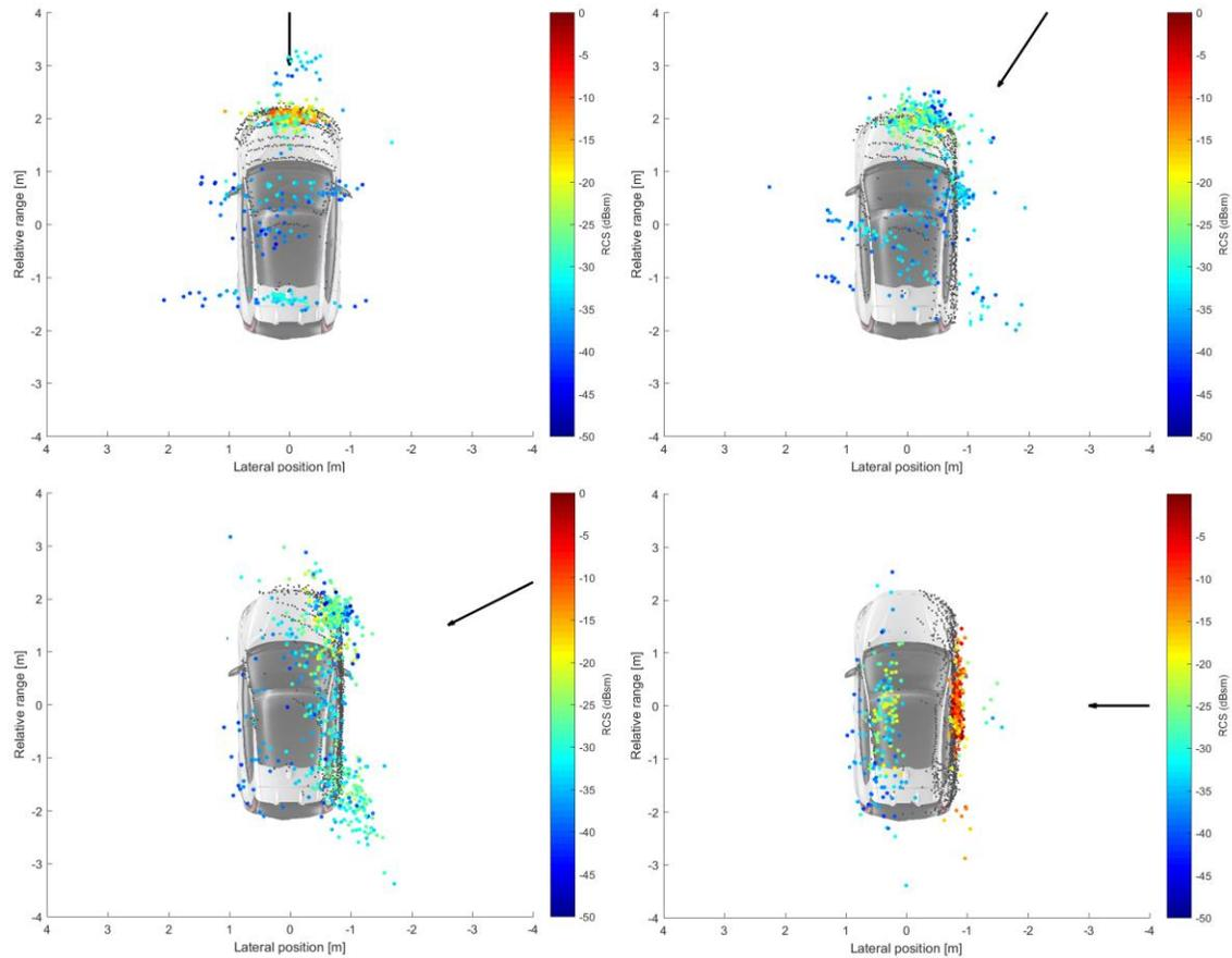
Figure 12. Back projected detections overlaid on a lidar point cloud of a Volvo V40 for four different approach angles. The upper left is an approach at  $0^\circ$ , the upper right at  $30^\circ$ , lower left at  $60^\circ$  and the lower right at  $90^\circ$ . The grey points overlaid on the image of the target are the point cloud from the Velodyne HDL64 lidar.
