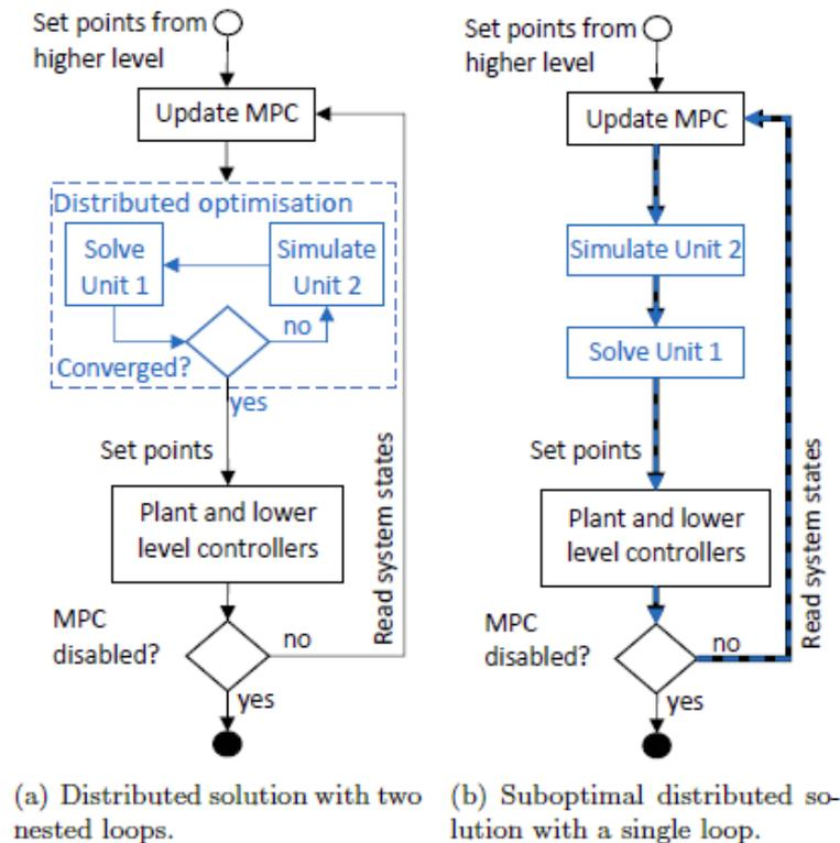
Figure 24 Decentralized control flow chart
