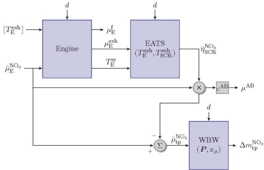
Figure 15 Complete supervisory control scheme
