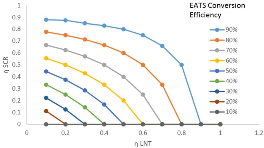
Figure 18 LNT-SCR NOx conversion efficiency for target EATS NOx conversion efficiency
