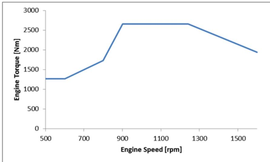
Figure 3 TC Engine speed-torque curve
