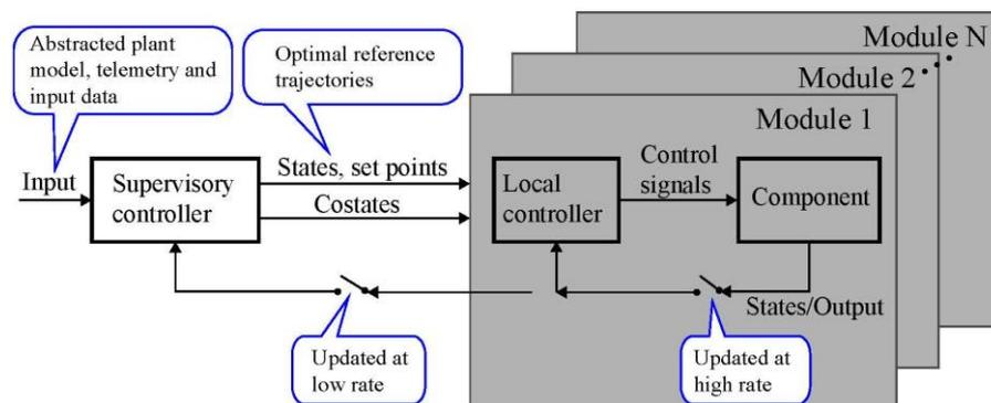
Figure 9 Modularized control system
