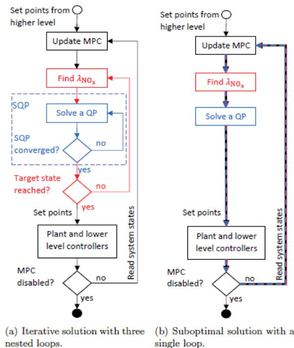
Figure 23 Centralized controller flow chart
