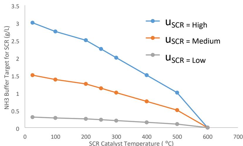
Figure 21 Target ammonia buffer in the SCR modified by introducing the SCR supervisory control parameter  $u_{SCR}$
