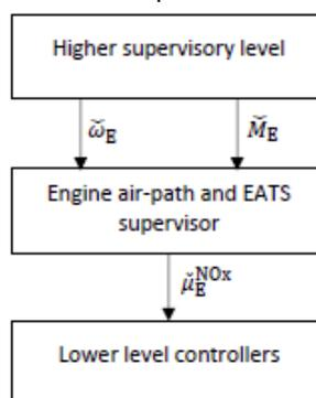
Figure 22 Hierarchical architecture for NO<sub>x</sub> emission control
