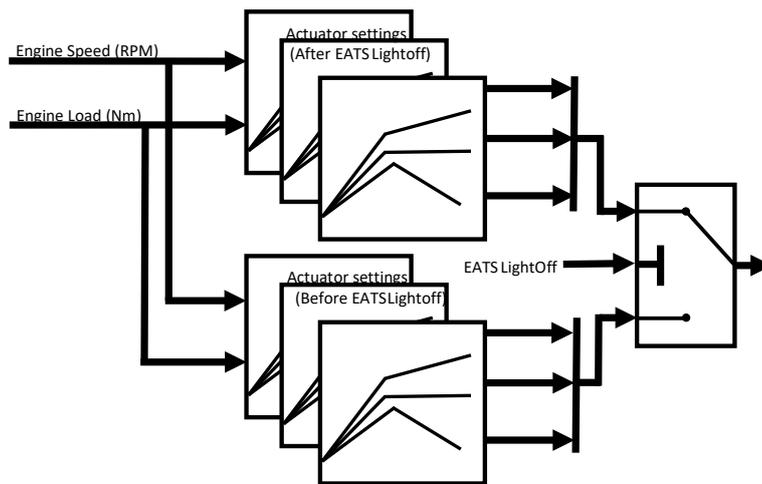
Figure 25 Baseline controller for light duty applications
