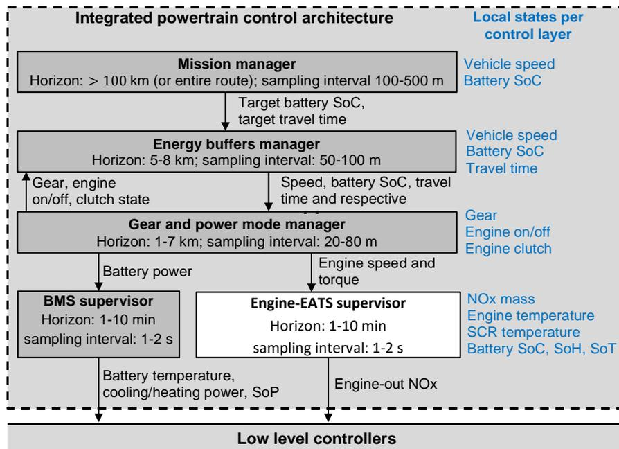
Figure 10 Layered control system architecture
