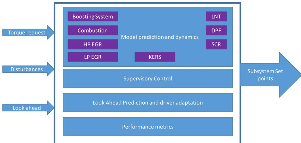
Figure 16 Supervisory control for light duty applications
