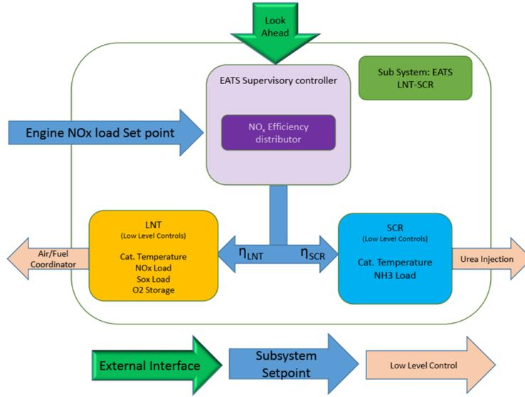
Figure 19 Supervisory control structure indicating signal flows and interface between the supervisory controller, the local controller and the actuators
