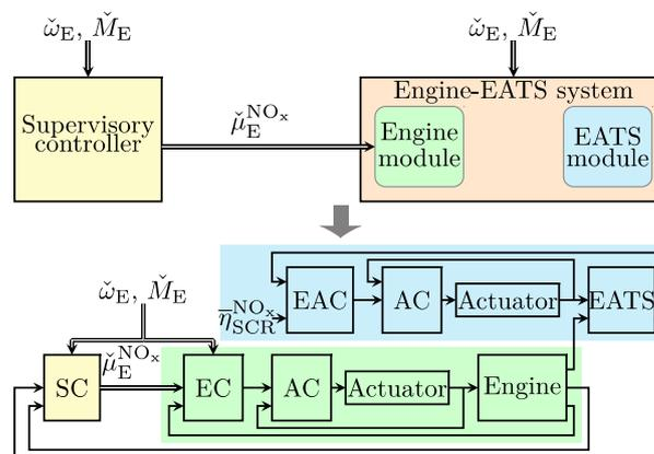
Figure 11 Detailed supervisory control scheme
