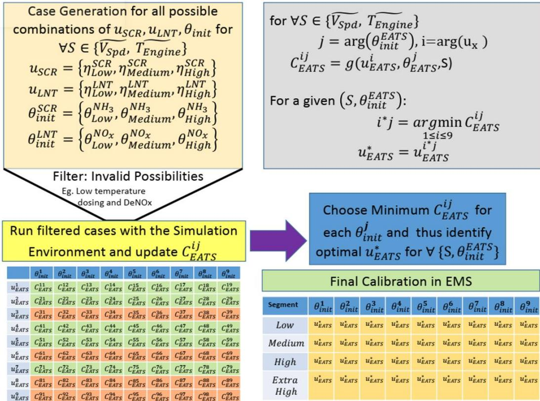
Figure 20 Visualization of the optimization methodology for light duty applications
