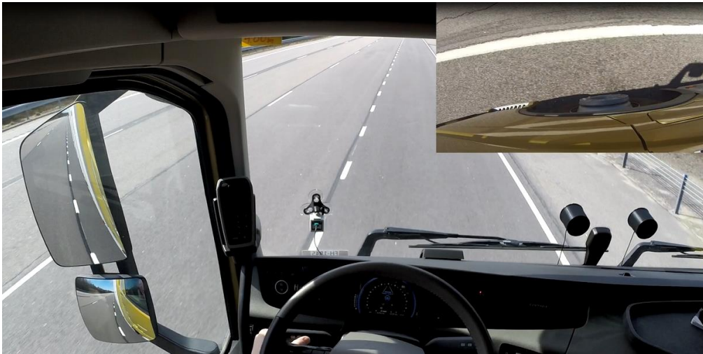
Figure 14 A golden truck at a test track to evaluate lateral control. Right corner: top view of front right wheel.
