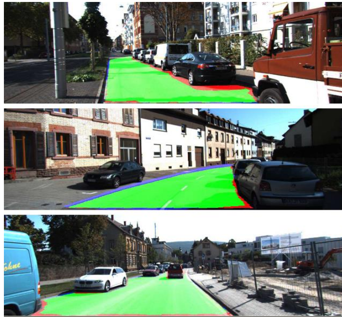
Figure 8 Examples of road detection in images view. Green denotes true positive, red and blue correspond to false negative and false positive respectively.
