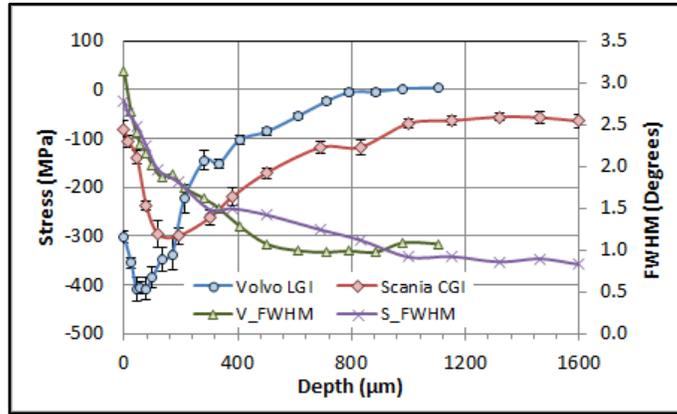
Figure 3. Residual stress and FWHM profiles in blasted LGI and CGI.  $XEC=5.81 \times 10^{-6} \text{ MPa}^{-1}$
