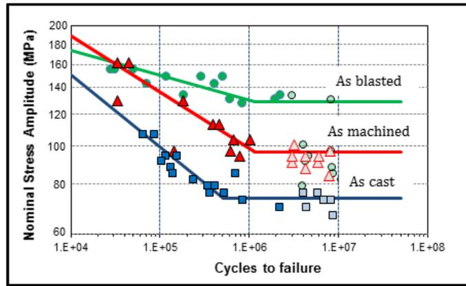
Figure 4. S-N curves for Volvo LGI. Stress ratio R ratio = 0.1, runouts: over  $3 \times 10^6$  cycles.
