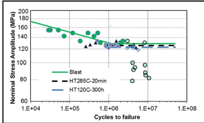
Figure 6 The effect of heat treatments on Volvo blasted LGI. R ratio=0.1, runouts: over  $3 \times 10^6$  cycles.
