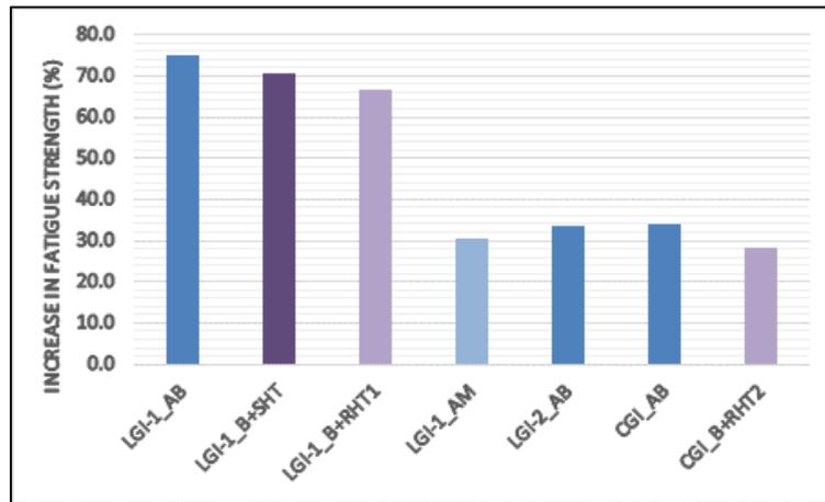
Figure 1. Improvement in fatigue limit after the different treatments. AB: as blasted, AM: as machined, B+SHT: blasting + annealing 20 min at 285 °C, RHT1: blasting + annealing 300 h at 120 °C, RHT2: blasting + annealing 300 h at 220 °C.
