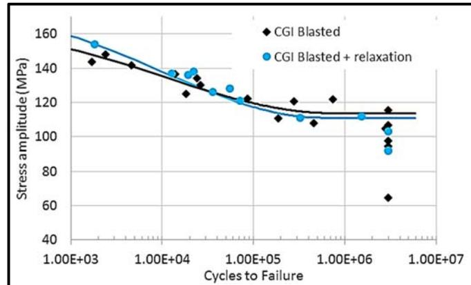
Figure 7 The effect of stress relaxation annealing (300 h at 220 °C) on Scania blasted CGI. R ratio= $\sim 0.15$ , Runouts: over  $3 \times 10^6$  cycles.
