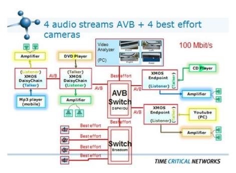
Figure 4: AVB Sound and regular video (2nd version of test bench)
