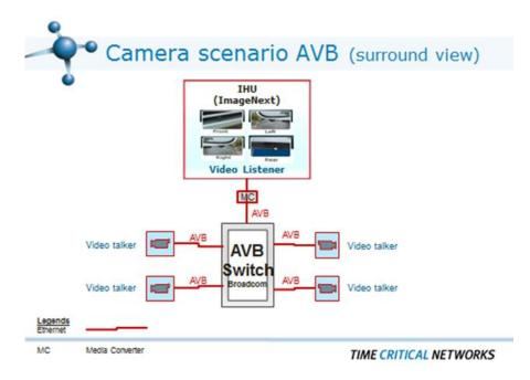
Figure 5: AVB Video only (3rd version of test bench)
