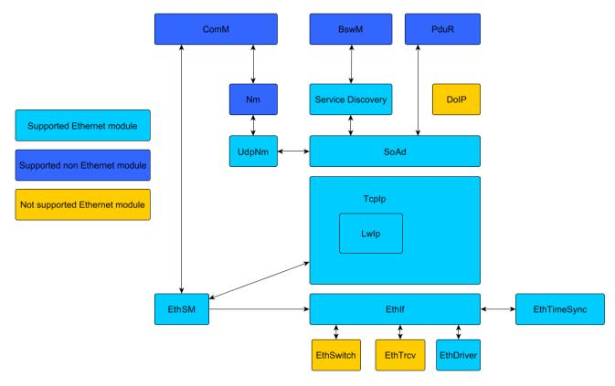
Figure 6: AUTOSAR 4.2 Ethernet stack overview
