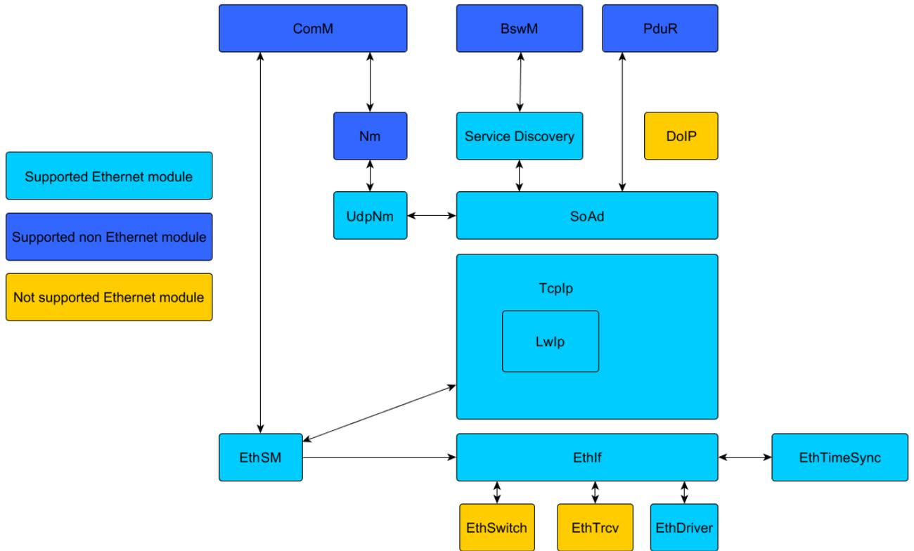
Figure 6: AUTOSAR 4.2 Ethernet stack overview
