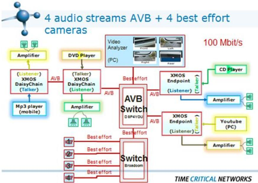
Figure 4: AVB Sound and regular video (2nd version of test bench)
