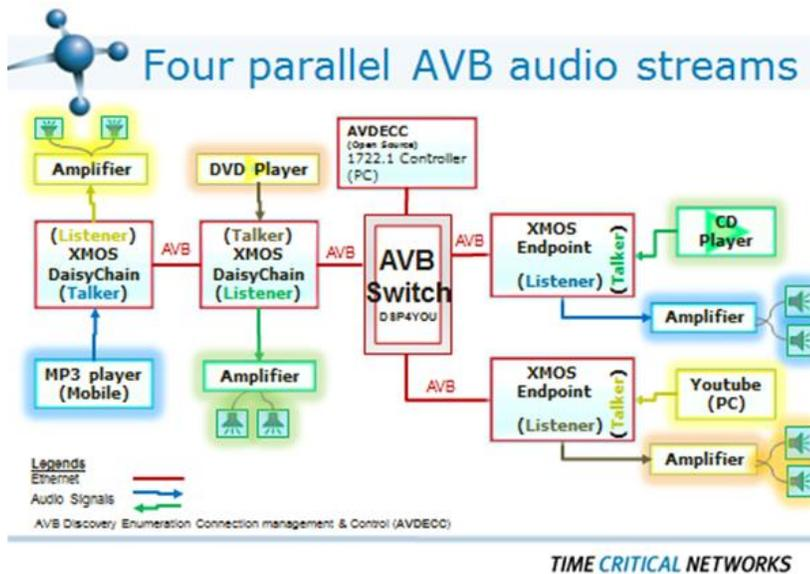
Figure 3: AVB Sound only (1st version of test bench)
