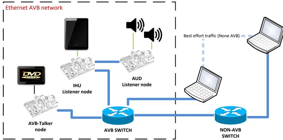
Figure 2: An example AVB network showing an infotainment domain use case
