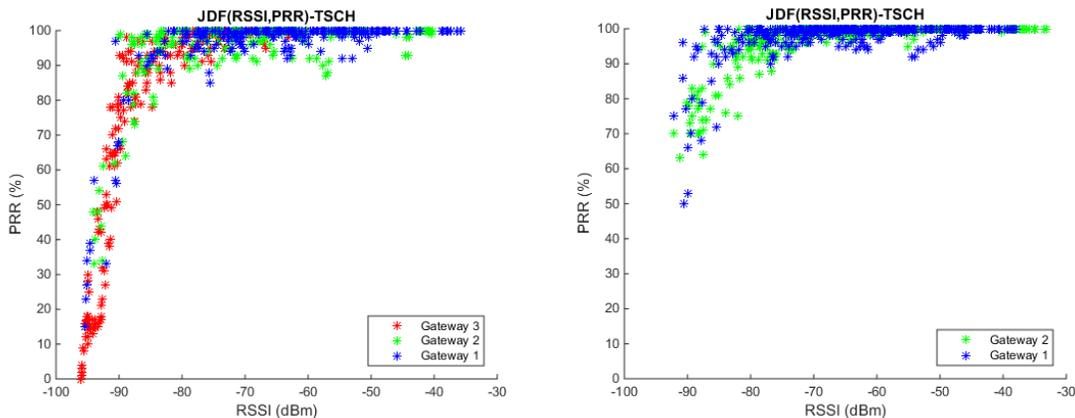
**Figure 5 - A joint distribution of packet reception rates and received signal strengths (a) FH 6x2 tractor and (b) FH 6x2 tractor with a semi-trailer**
