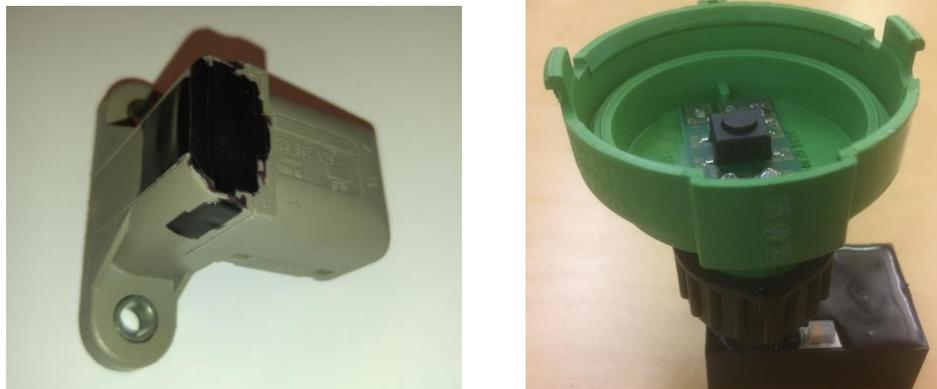
Figure 7 - Prototype battery powered cab-tilt lock switch (left) and air-filter pressure switch (right)
