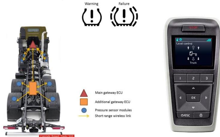
Figure 1 – Tire Pressure Monitoring System (left) and ECS4 Work remote for a Volvo FH (right) which use short-range wireless communication
