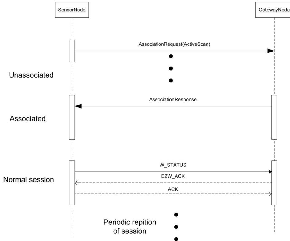
**Figure 3 - Application protocol for sensors**
