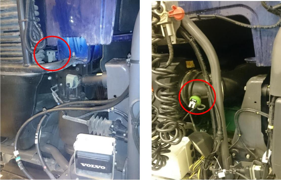
Figure 10 - Installation of cab-tilt lock (left) and air-filter pressure (right) switches
