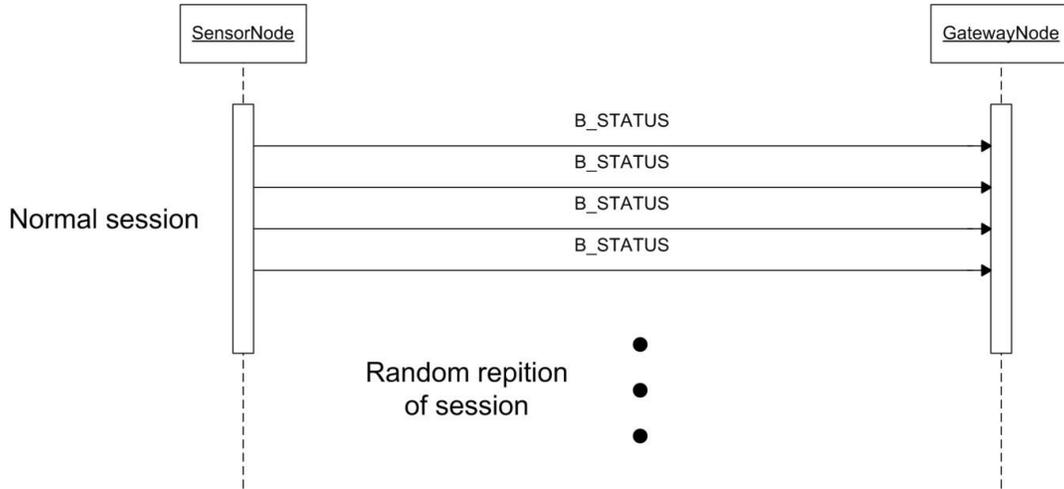
Figure 4 - Application protocol for switches
