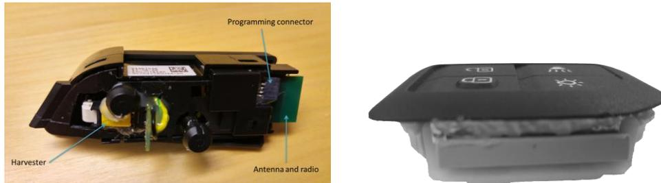
Figure 6 - Prototype energy harvesting city horn switch (left) and energy harvesting keyfob (right)
