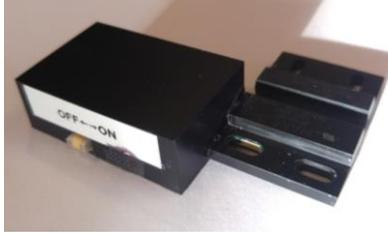
Figure 8 - Trailer door lock switch
