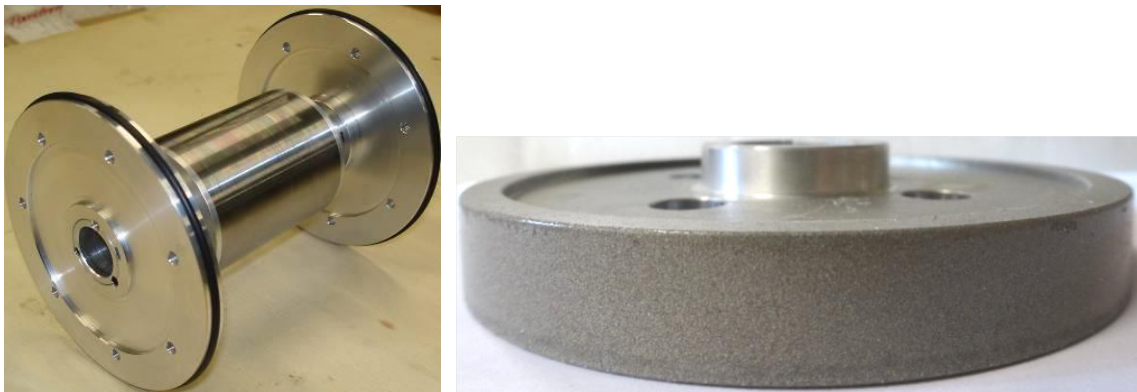
Figure 2. Left Wheels with o-ring in a slot; Right Friction wheel coated with friction material.
