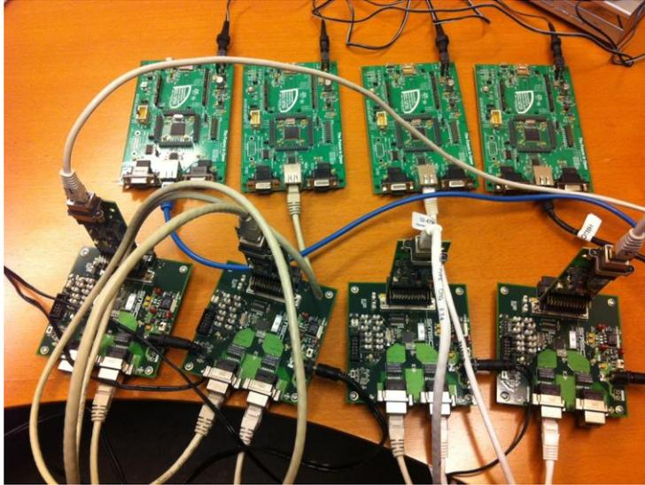
Figure 7: Example of test setup with prototype ECUs
