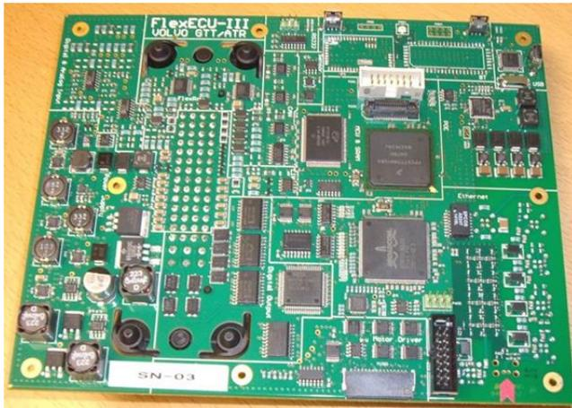
*Figure 2: Photo of FlexECU-III printed circuit board*
