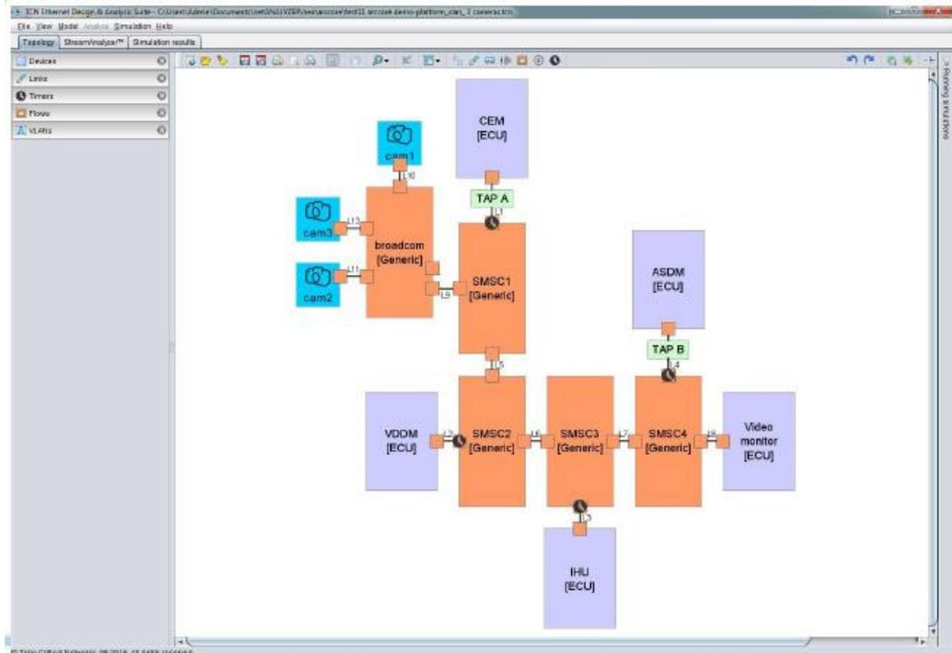
Figure 4: Example Input to Simulation – Video streams from cameras
