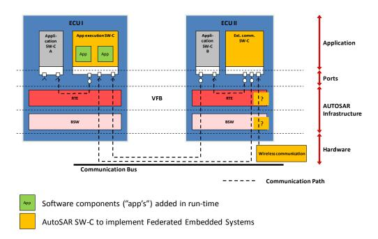
The objectives of the project were to develop the AUTOSAR software components for plug-in execution and external communication, and validate them in a realistic setting. Also, supporting tools were to be considered.
