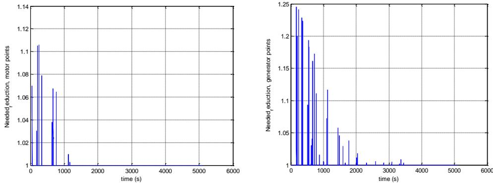
Figure 6: Derating at motoric (left) and regenerating (right) operation in order to avoid over voltage.
