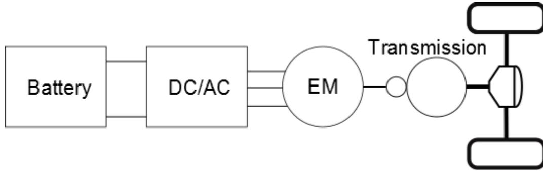
Figure 1: Main circuit components for electric propulsion of a vehicle. Battery, converter, with its dc-link capacitor and 6 transistors, gear and wheel pair.
