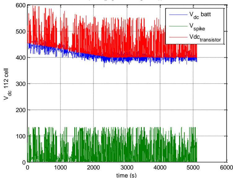
Figure 3: Battery voltage, **blue**, dc voltage in the inverter, **red**, size of switching transients, **green**, for the drive cycle operation, with 15 % more battery cells.
