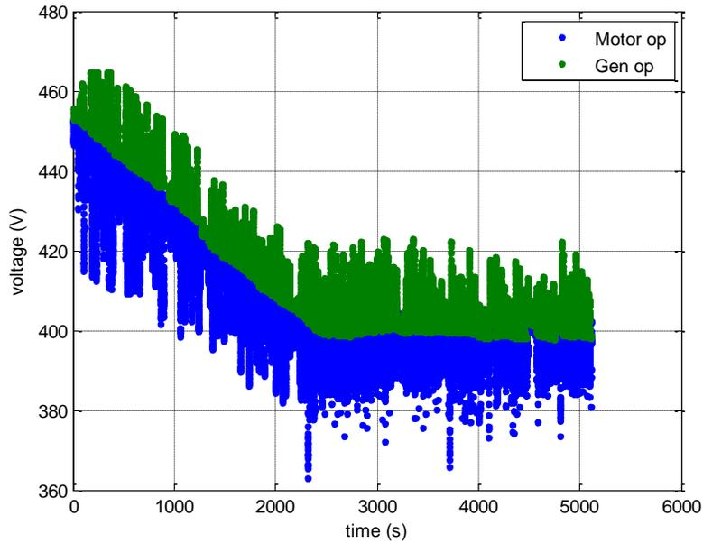
Figure 4: Battery voltage for a drive cycle operation, with 15 % more battery cells.
