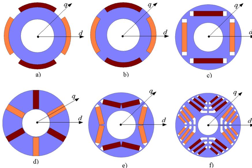
Figure 8: Rotor topologies for permanent magnet machines with varying degree of saliency.
