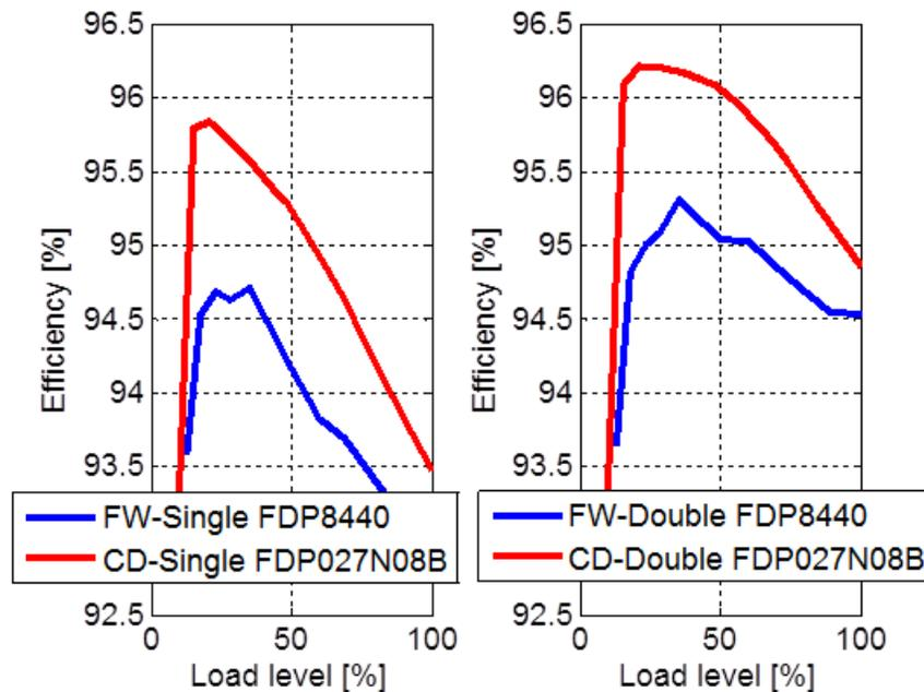
Figur 10: Efficiency of the two topologies, blue fullbridge converter red, current doubler, left, single power semiconductors, right – double semiconductor components on the secondary side.
