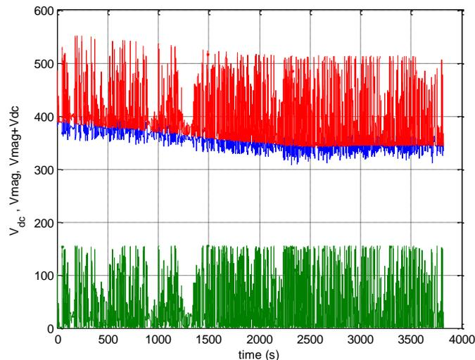
Figure 2: Battery voltage, **blue**, dc voltage in the inverter, **red**, size of switching transients, **green**, for the drive cycle operation.
