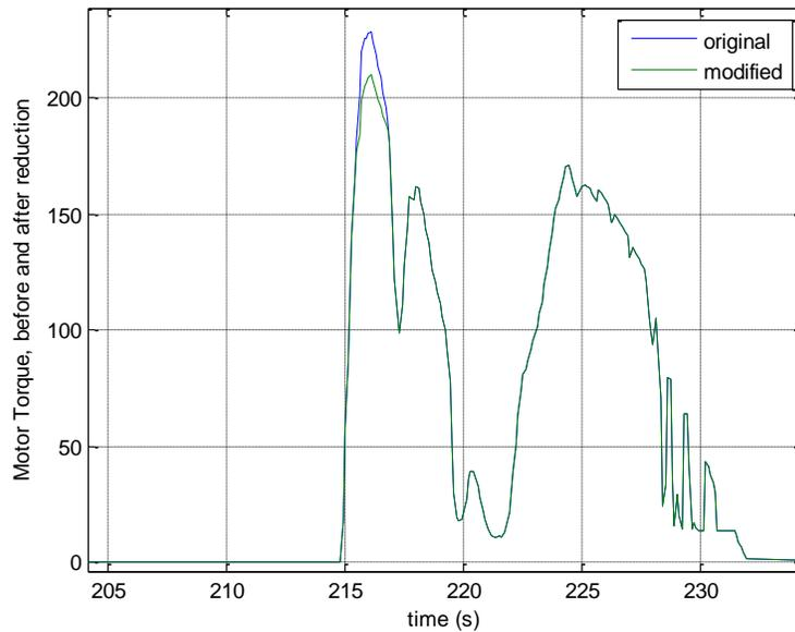
Figure 5: (Torque) derating at a propulsion event during the drive cycle..
