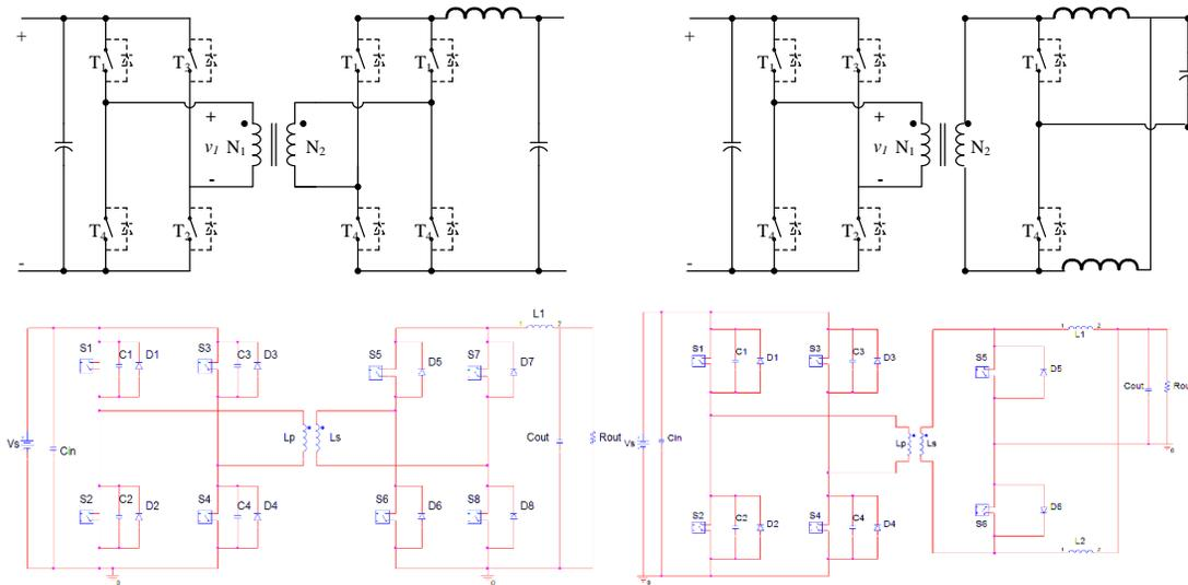
Figure 9: Secondary side converter topologies: On the left, a full bridge layout and on the right a current doubler.
