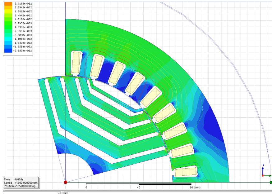
Figure 7: Cross-section of the synchronous reluctance machine model.
