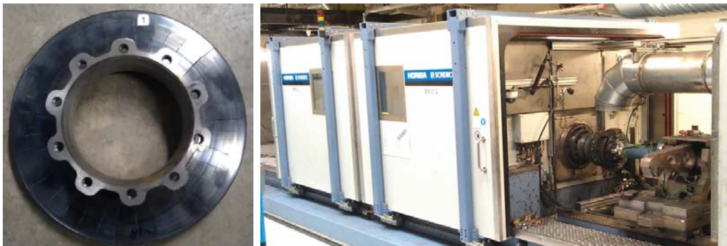
Figure 1. Disc with severe cracking (left) and overview of the full scale brake dynamometer (right).
