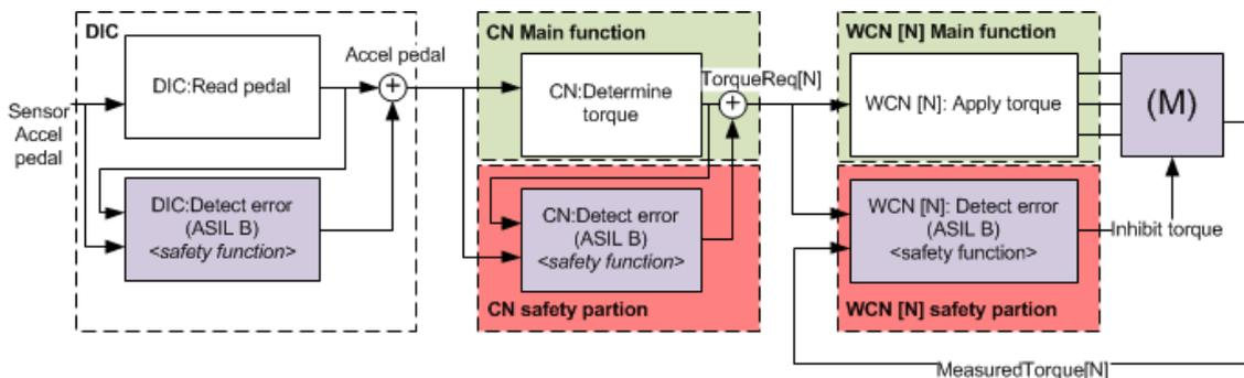
Figure 15 – Example of Functional Safety Concept allocation (Safety Goal 1)
