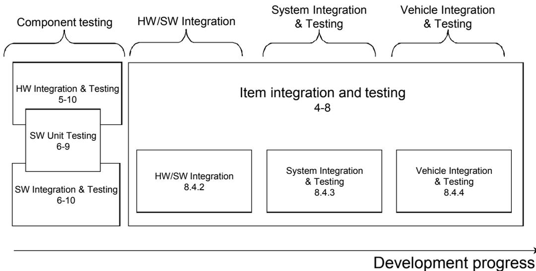
Figure 5. In the picture references is made to different parts of the ISDO26262 standard, giving guidelines for different levels of testing.
