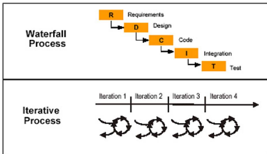
Figure 4 Waterfall model is normally suitable for non- complex system development and an Iterative development process more suitable for a more complex system development.
