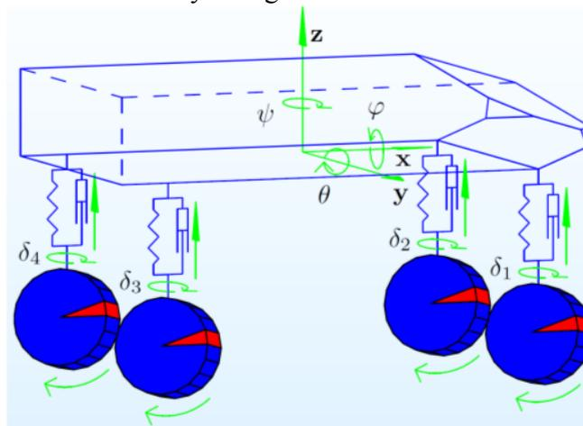
Figure 16 – Vehicle model with 18 degrees of freedom.
