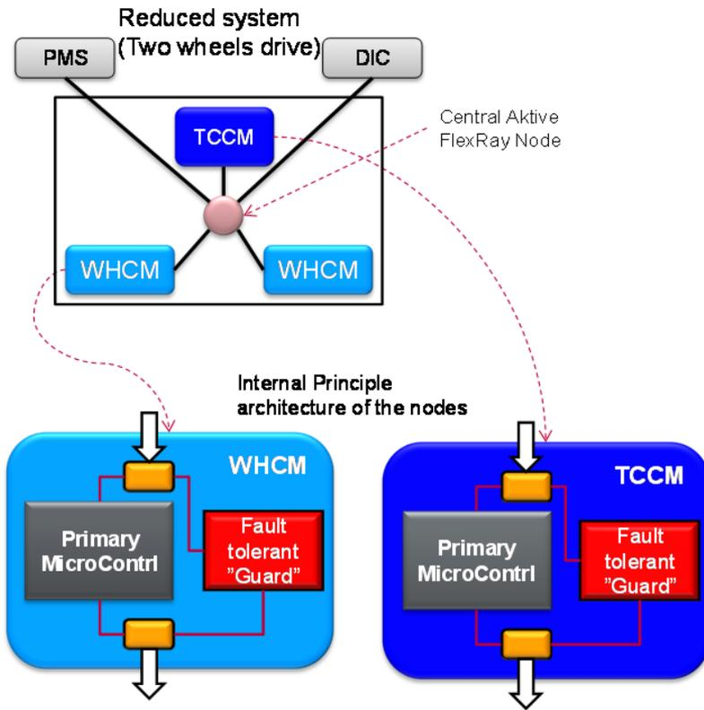
Figure 7. The use of multi core processors the probability for fault findings increases. By using the same principle design of the nodes investment in quality and reduction of price could be combined.
