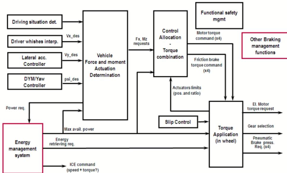
Figure 9 - Illustration of preliminary design for Electric Transmission Control Functional Architecture, final version (Red marked blocks are out of project scope)
