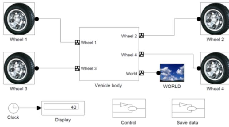
Figure 18 – Implementation of vehicle model in SimMechanics.
