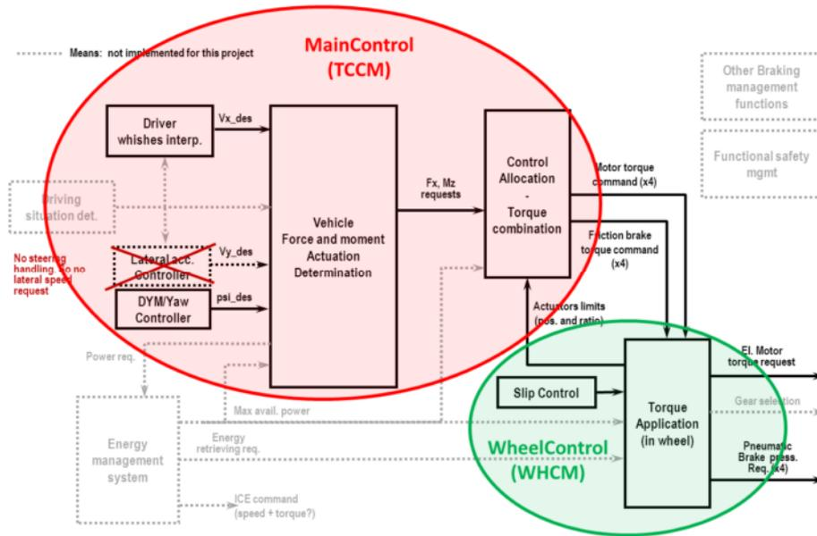
Figure 12 - AFFE functions repartition in functional components
