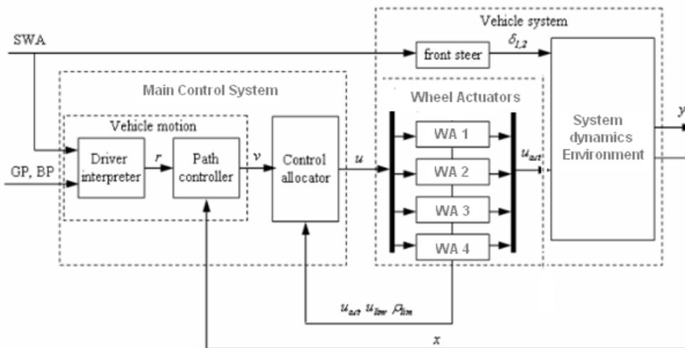
Figure 13 - Illustration of how Control system is. Used abbreviations in illustration: Steering Wheel Angle (SWA), Brake Pedal (BP), Gas Pedal (GP), Wheel Actuator (WA)
