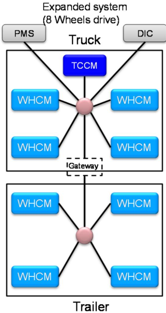
Figure 8. The use of FlexRay communication net could be expanded to cover also a trailer supporting the transmission with additional hub-motors. In the picture the network could be expanded with a redundant additional network that is supported by the FlexRay technology.
