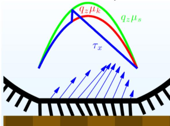
Figure 17 – Principle of the brush tyre model.
