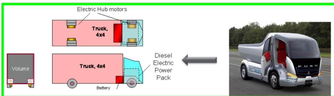
Figure 3. A typical Truck with four wheel serial hybrid drive was selected as a target system.
