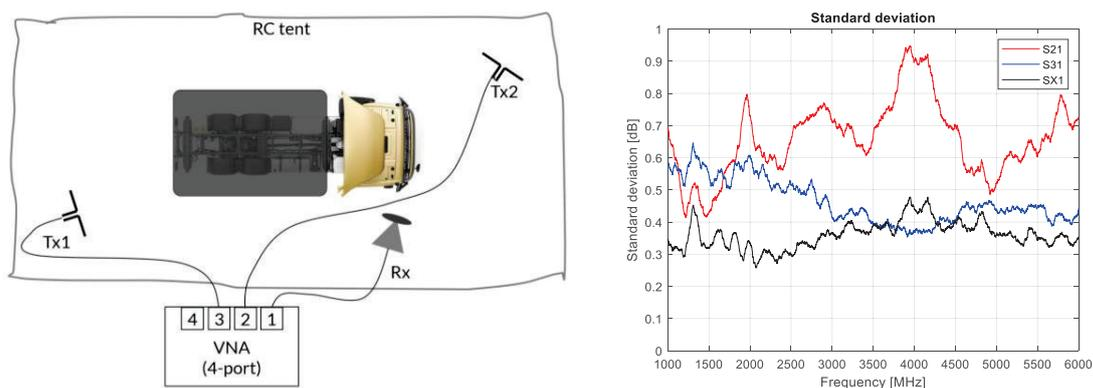
Figure 10. Measurement setup (left) and standard deviation (right) of individual Tx to Rx sets ( $s_{21}$ , or  $s_{31}$ ), and the combination of the two ( $(s_{21} + s_{31})/\sqrt{2}$ ).
