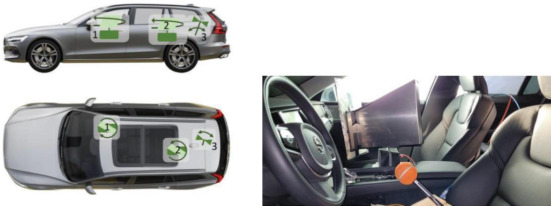
Figure 18. Left: Overview of ROBT stirrers: (1) clockwise mode stirrer, (2) counterclockwise mode stirrer, (3) Tx antenna placed on oscillating stand. Right: Continuously clockwise rotating stirrer (1) placed in front passenger seat.
