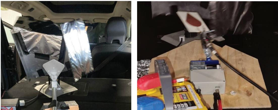
Figure 19. Left: Counterclockwise stirrer placed in trunk (2). Right: Antenna oscillator. Oscillating the antenna back and forth from the left to the right (3).
