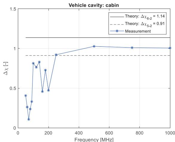
Figure 22.  $\Delta\chi$  close to the centre stack in a vehicle cabin. The cavity fulfils the stringent criterion from approximately 250 MHz.
