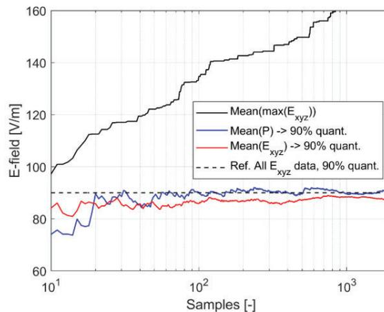
Figure 6. The mean of electrical field maximum values (x, y, and z components) (black) compared with the predicted 90% test level based on the average power (blue), and on the average electrical field (red). The reference (black dashed) is the 90% highest electrical field of the entire dataset (including x, y, z components).
