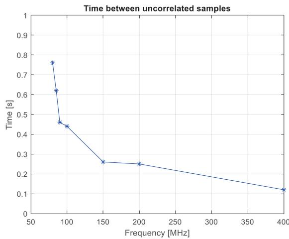
Figure 7. Time between samples in RC tent based on autocorrelation and  $1/e$  limit as function of frequency.
