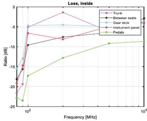
Figure 13. Field into trunk and different positions in car cabin. Mean total electrical field in specific position normalized with mean total electrical field in reference position outside vehicle.
