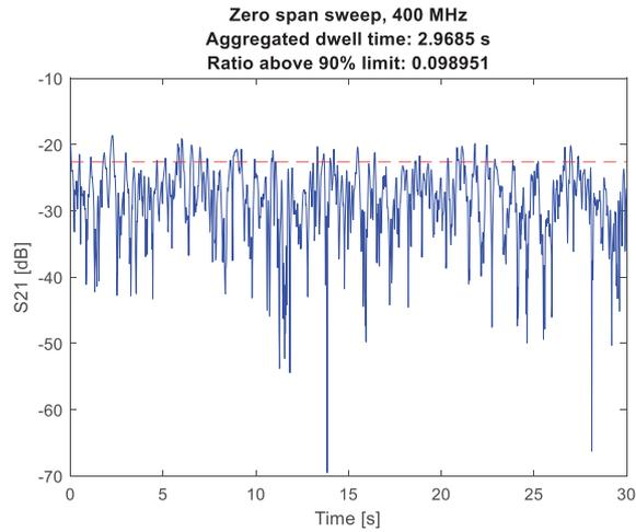
Figure 9. Zero-span sweep with calculated aggregated dwell time at 400 MHz.
