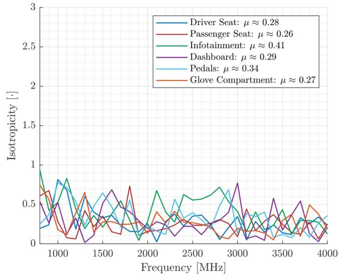
Figure 23. Isotropy in different positions. Figure from [5].
