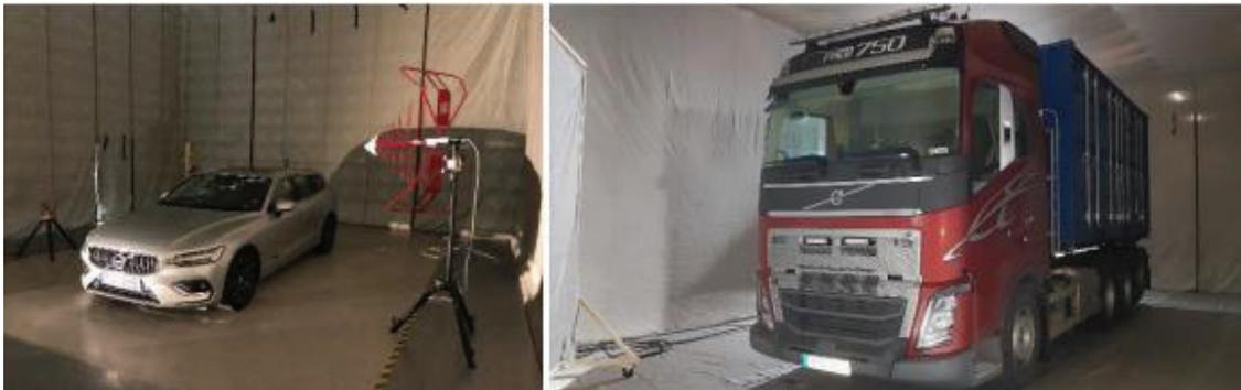
Figure 1. Vehicles during RF-immunity test in RC-tent (VIRC).
