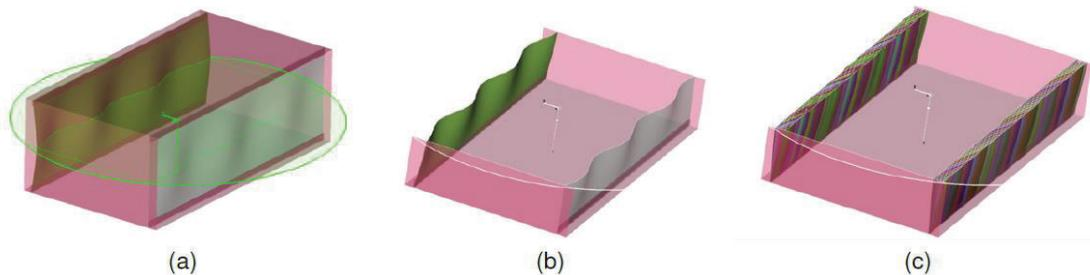
Figure 16. Visual representation of the VIRC simulation domain and model of the moving walls used in [4]. (a) One wall configuration. (b) Using a horizontal clip plane. (c) Showing all wall configurations at once.
