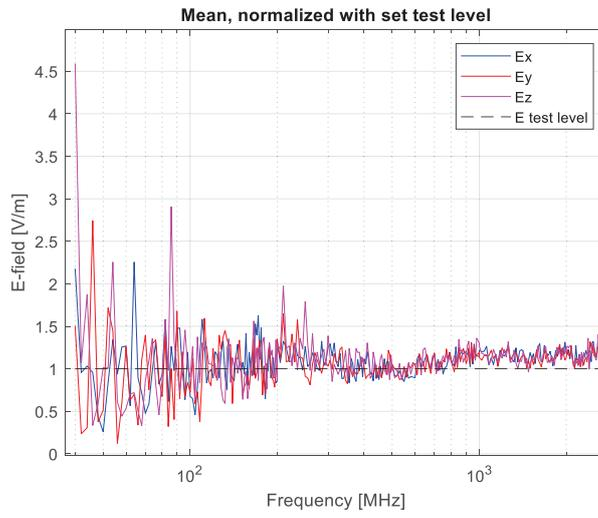
Figure 3. Mean of sampled fields, normalized with set test level (e.g., 100 V/m).
