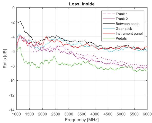
Figure 14. Field into trunk and different positions in car cabin.
