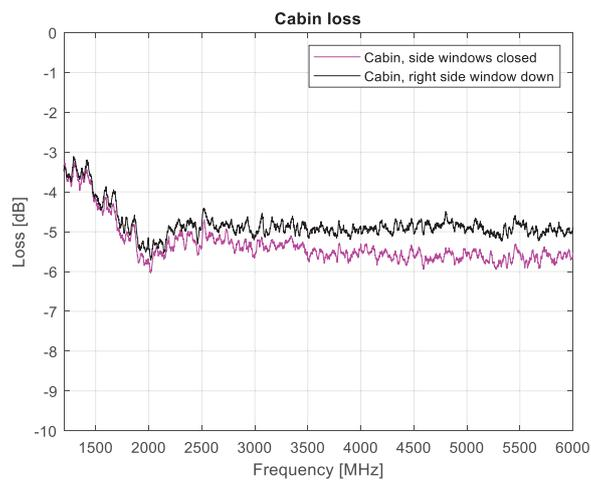
Figure 15. Field into truck cabin. Windows closed, or right-side window open.
