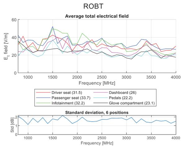
Figure 26. Average total electrical field in six different positions and standard deviation between these six datasets. Numbers in parenthesis are average values per position.
