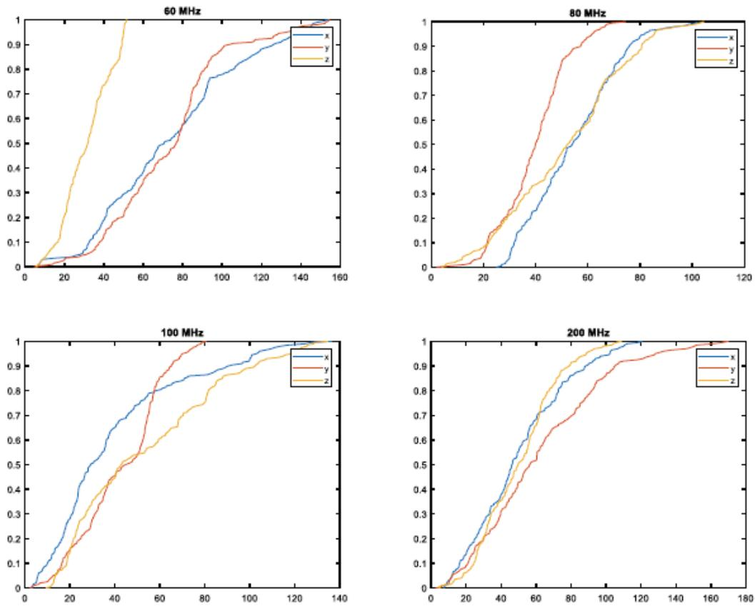
Figure 4. CDFs of electrical field (x-, y-, and z-components) at different frequencies. At 60 MHz there is no Rayleigh distribution, and at 200 MHz data is Rayleigh distributed.
