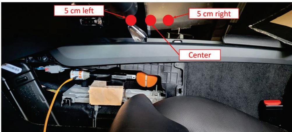
Figure 28. Positions of the OBT antenna. All three positions were tested in V-pol (antenna elements parallel to driving direction of vehicle) and H-pol (antenna elements perpendicular to driving direction of vehicle).
