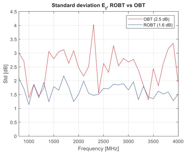
Figure 27. Standard deviation for the ROBT vs the standard OBT method. Averages in parentheses.
