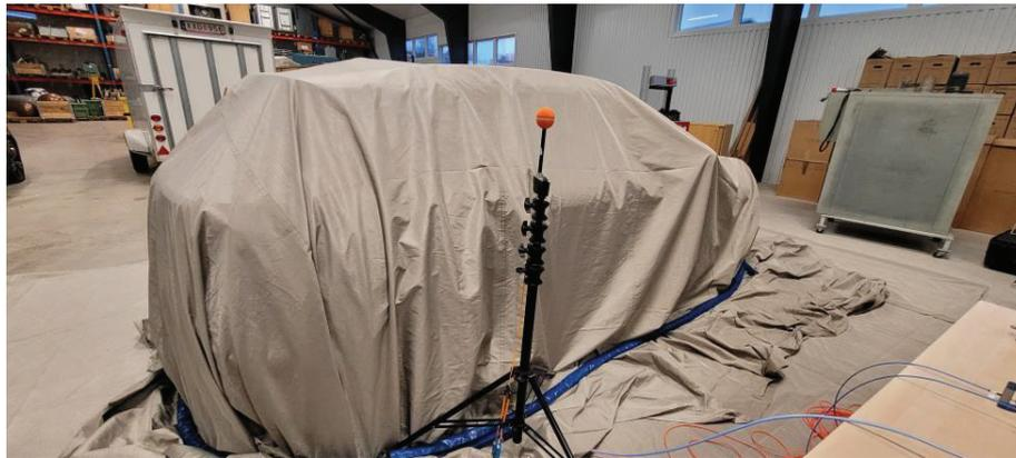
Figure 17. VUT covered by conductive textile sheets for ROBT testing. A probe is here placed outside the VUT for shielding verification measurements.
