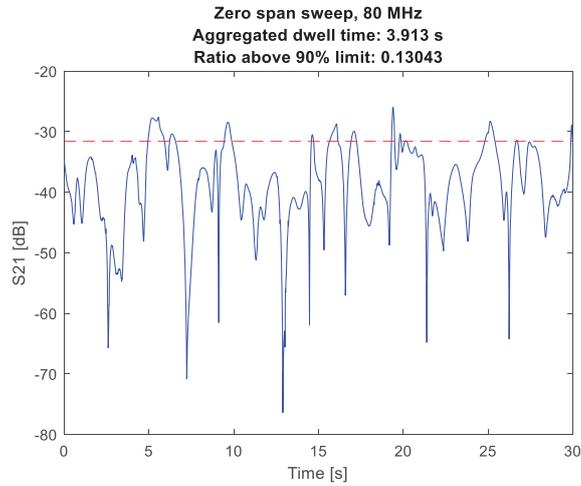
Figure 8. Zero-span sweep with calculated aggregated dwell time at 80 MHz.
