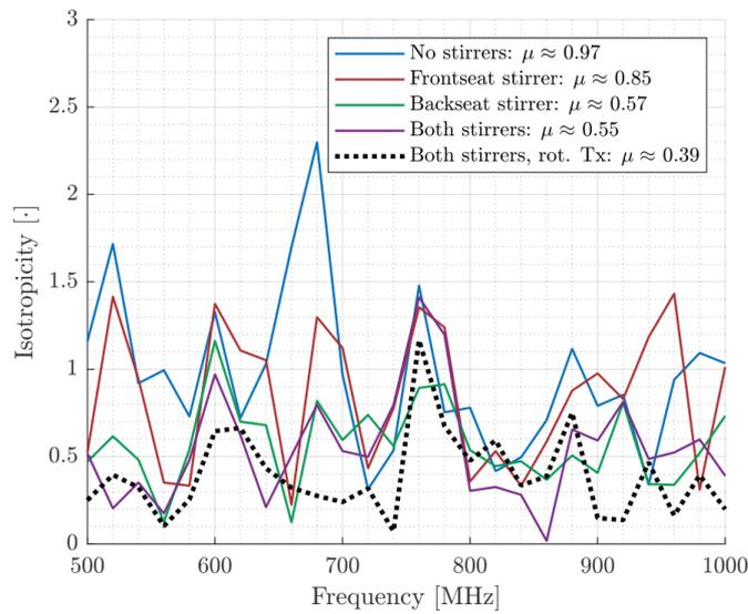
Figure 20. Isotropy over frequency for different stirrer settings. Figure from [5].
