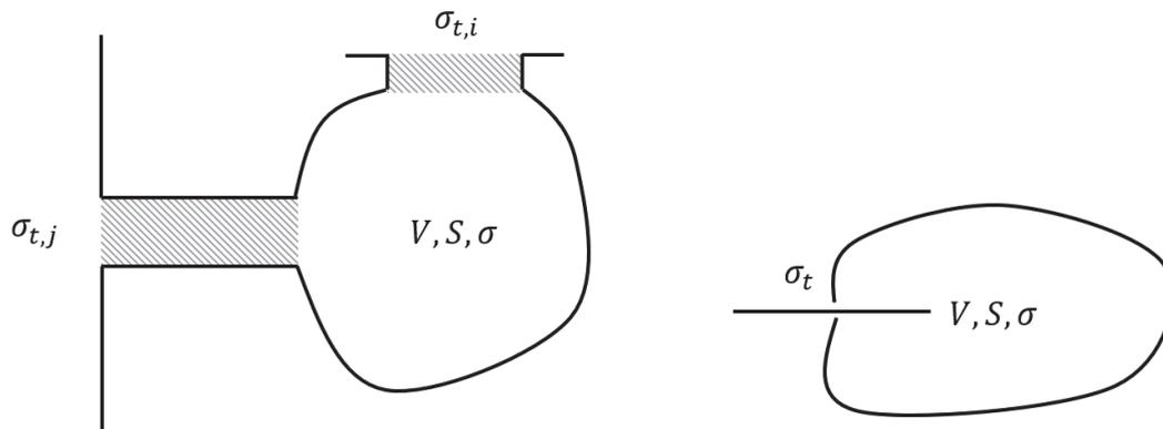
Figure 11. Left: a cavity with two apertures (grey). Right: A cavity punctuated by conductive wire.
