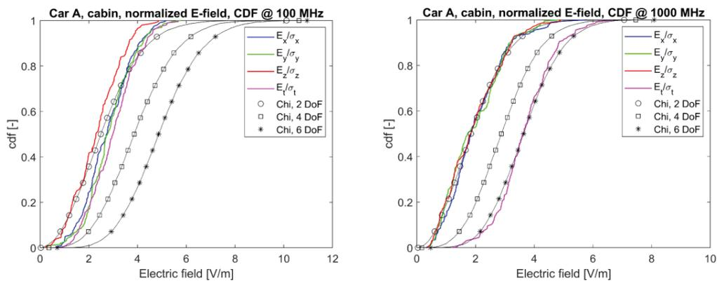
Figure 12. CDF of normalized electrical field sampled in the cabin of car A. Left: at 100 MHz the total electrical field magnitude is  $\chi$ -distributed with less than two DoF. Right: The total electrical field magnitude is  $\chi$ -distributed with approximately six DoF.
