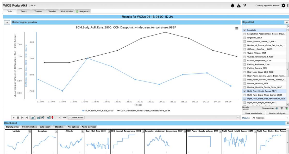
Figure 8: Screenshot of visualization of signals collected using PLA sampling. The line segments between the points are the linear approximations, where multiple data points would have been present using conventional sampling.
