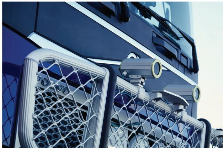
*Figure 19. Cameras mounted on the test vehicle.*
