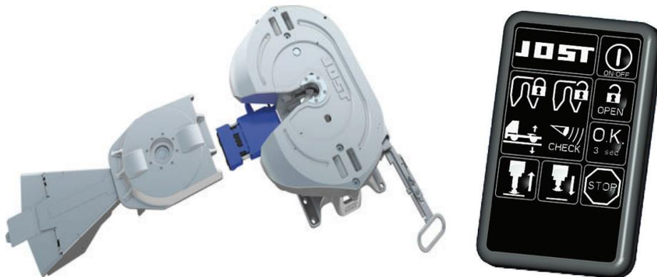
*Figure 13 – Trailer unit with king pin and fifth wheel for the KKS system (left). The blue part is the automatic connector for air and electrical supply, mating with the triangular part on the trailer side when coupling the semi-trailer. Control panel in cabin for the KKS system (right).
