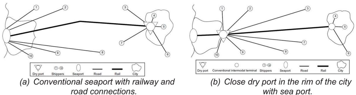
Figure 3. Conventional sea port layout (a) compared with a close dry port connected by electric railway (b) (Roso, et al. 2009).
