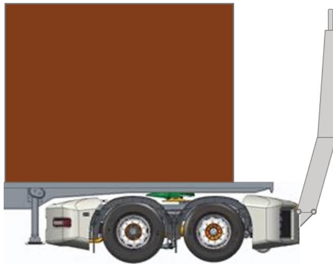
*Figure 12. Illustration of iDolly with foldable drawbar.*
