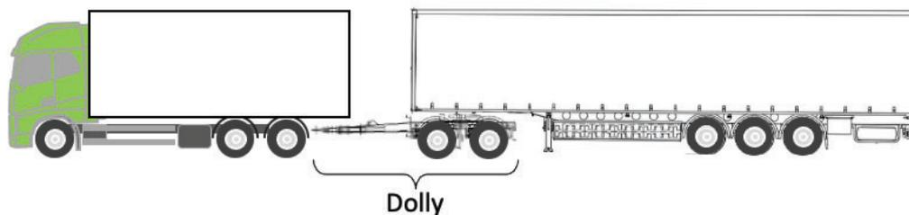
*Figure 1. A dolly used to connect a semi-trailer to a rigid truck in a 25.25m long “Nordic combination”.*
