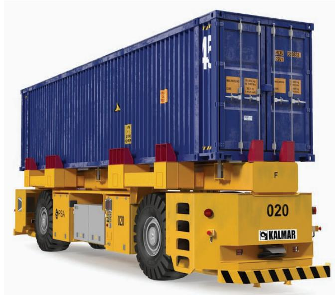
Figure 6. An AGV for transport of containers (courtesy of Kalmar Industries).
