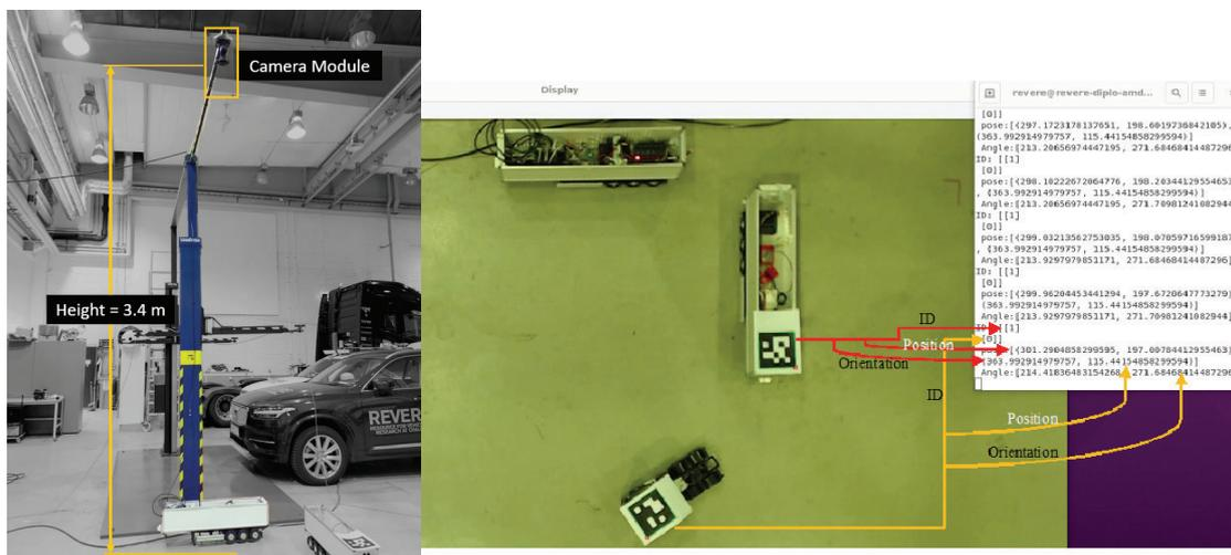
Figure 26. Overhead camera placement (left) and tracking using ArUco markers (right).
