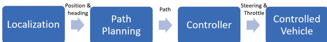
Figure 24. Basic building blocks for the reversing algorithm.
