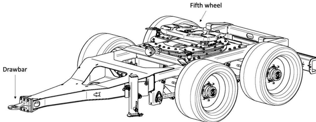
Figure 5. Converter dolly (courtesy of AutoComp AB).
