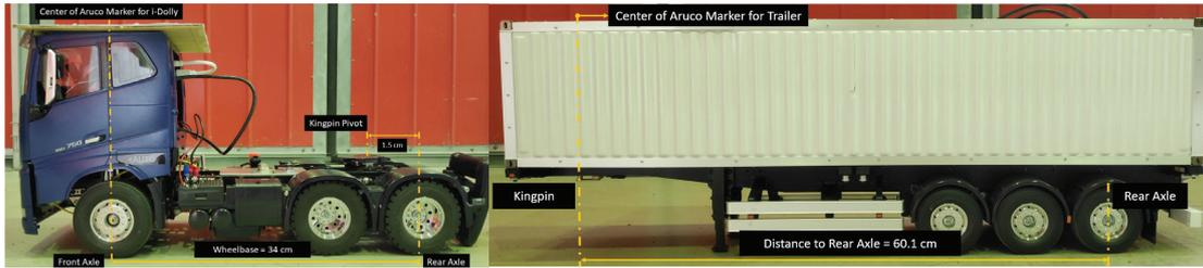
Figure 25. Scaled down model used for the test and demonstration
