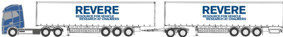
*Figure 4. The type of A-double combination studied in the Autofreight project. A 6x4 tractor is coupled with a semi-trailer, a dolly and a second semi-trailer.*
