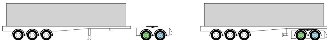
Semi-trailer and iDolly coupling / decoupling with changing height and landing gear lifting. iDolly acting on its own as a "master" unit.
