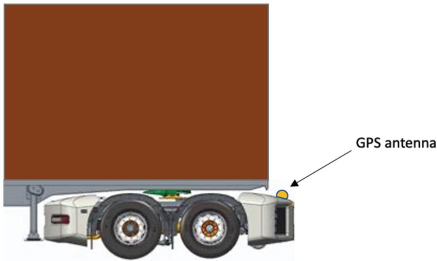
Figure 18. GPS antenna coverage partly occluded by trailer and (45 foot) container.
