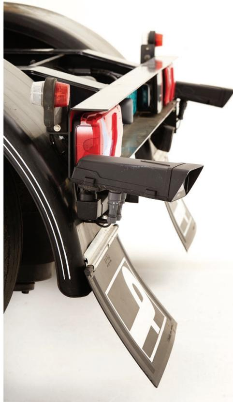
*Figure 21. Cameras mounted on the rear end of a dolly for testing camera views.*
