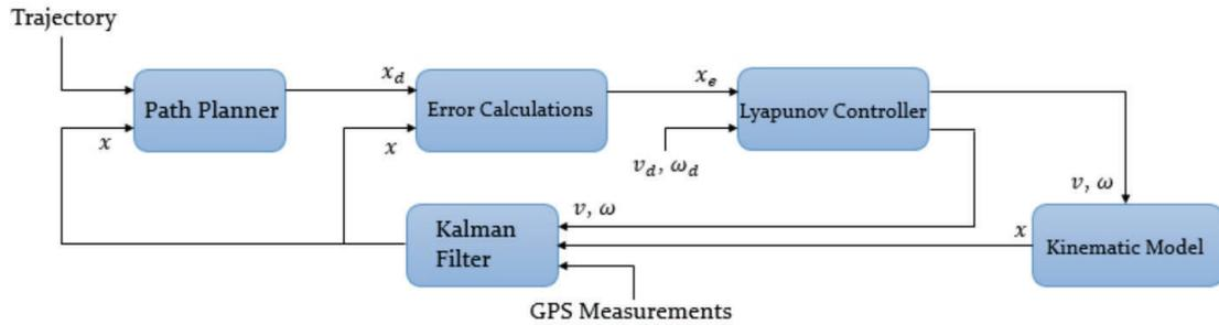
Figure 16. Overview of the complete system. The control signal  $x$  is the state vector that consists of  $x$  and  $y$  coordinates and the vehicle's heading  $\theta$ .
