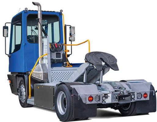
Figure 14. A Terberg terminal tractor with hydraulically liftable fifth wheel (courtesy of Terberg).
