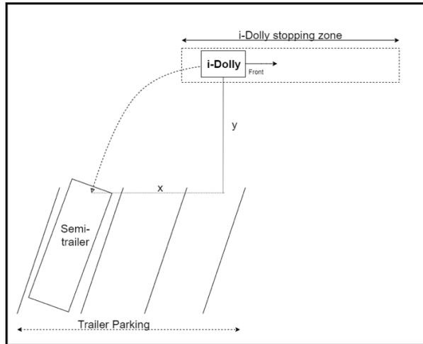
Figure 27. iDolly reversing to couple a semi-trailer.
