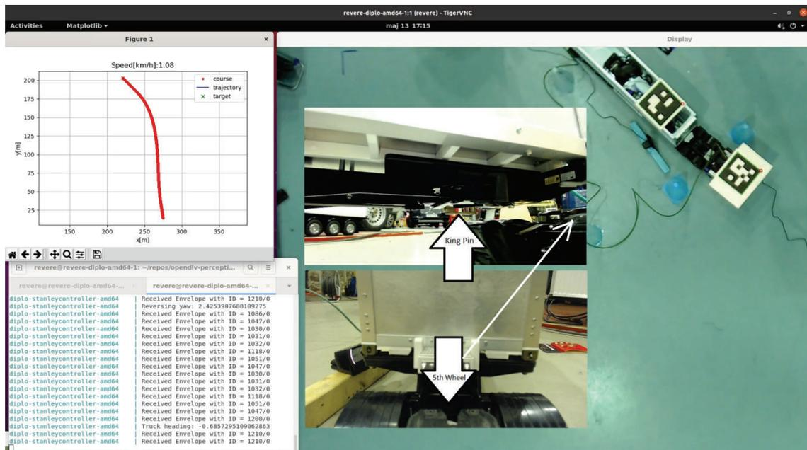
Figure 28. Different camera views showing the fifth wheel approaching the semi-trailer king pin.
