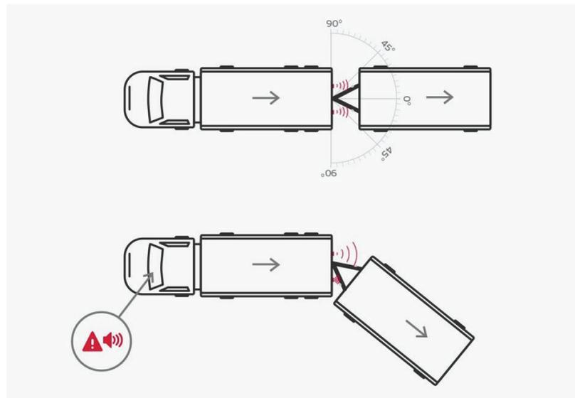
Figure 22. Radar system for drawbar angle measurement.
