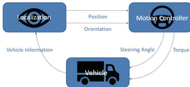
Figure 15. Overview of the interactions between the localization procedure, the motion controller and the vehicle. The position and orientation of the truck/iDolly is measured with respect to the trailer.
