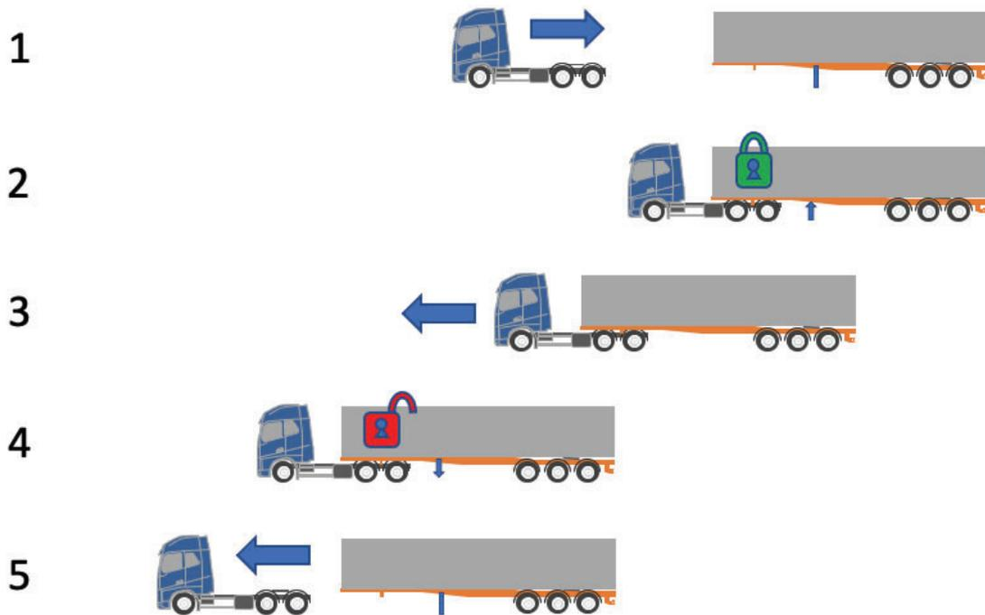
Figure 23. Demonstration of automated coupling and uncoupling of a semi-trailer.
