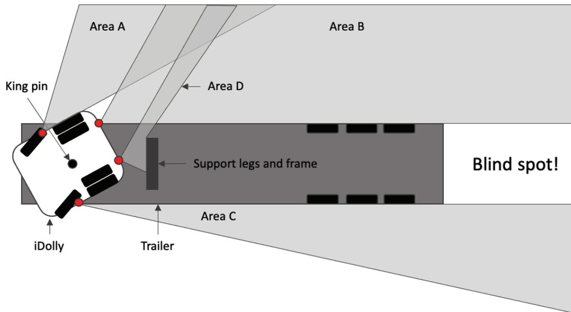
Figure 20. Illustration of camera coverage behind the iDolly when making a turn with coupled semi-trailer. Red dots illustrate camera positions.
