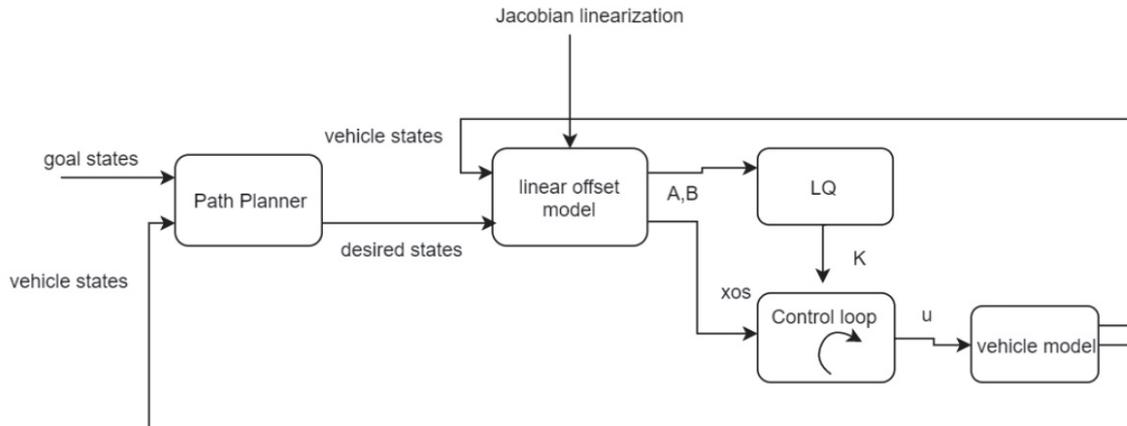
Figure 17. Complete control algorithm overview
