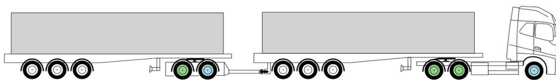
A-double combination vehicle with an eDolly acting as a "slave" unit.
