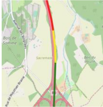
Fig. 9: Visualization of an aspect of predictive maintenance based on street quality and vehicle component status. This is a proof-of-concept. What is shown is a visualization of the quality of a road, based on external data. While this is a mock-up with hard-coded street quality data, data for wear and tear of some components can be accessed via the vehicle's CAN bus. Visualization is optional for this use case.
