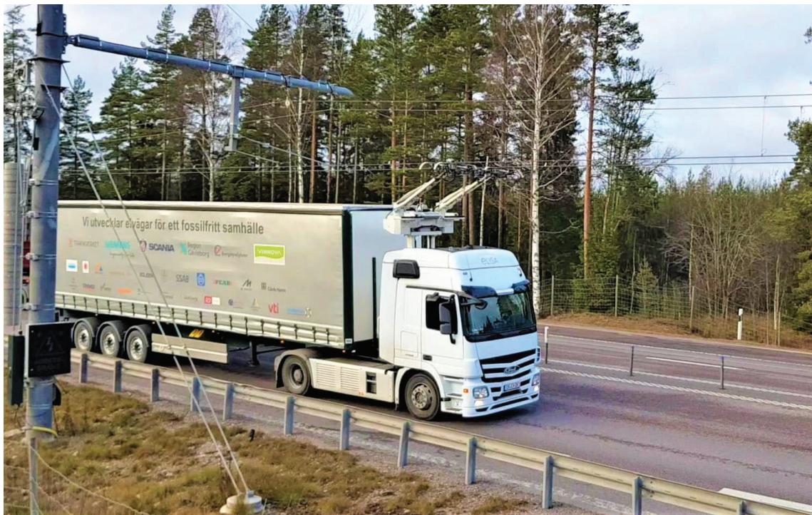
Figure 20: An eHighways truck with current collector on pantograph and overhead lines.
