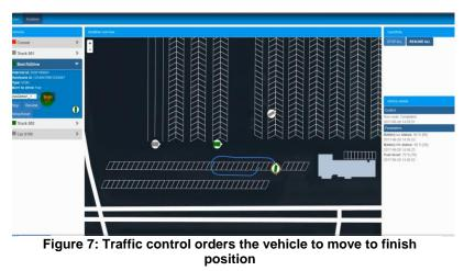
The vehicle executes the transport mission and remains in contact during the full flow with the traffic control. Dual handshake takes place to ensure that the vehicle will stop if there are any issues with connectivity. The movement of the vehicle is displayed in Figure 8.
