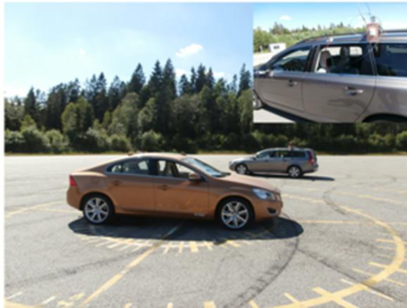
**Figure 34: Range Test object Volvo S60 in the middle of Skidpad and measurement vehicle driving around it following circle lines on different radiuses on the Skidpad. Upper right shows the measurement vehicle**
