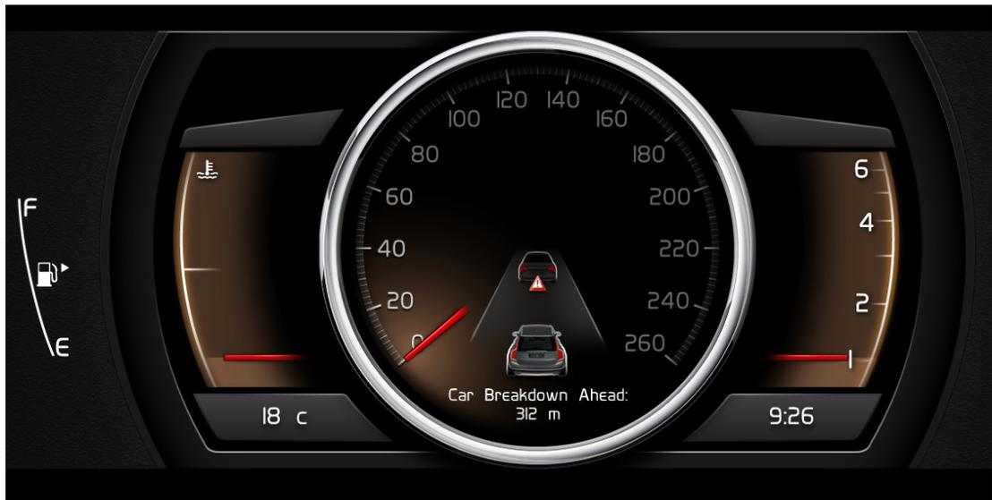
Figure 30: Stationary vehicle warning HMI in the ETTE Volvo car
