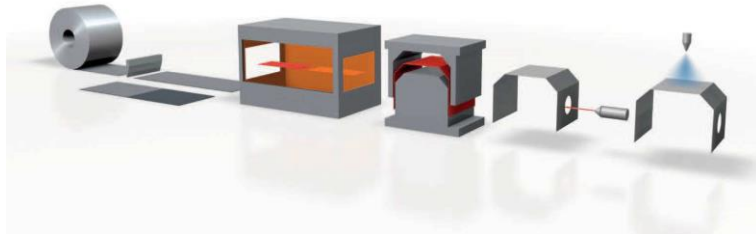
Figure 1: Schematic representation of the hot stamping process, from decoiling to finished product (image courtesy of voestalpine Steel division).
