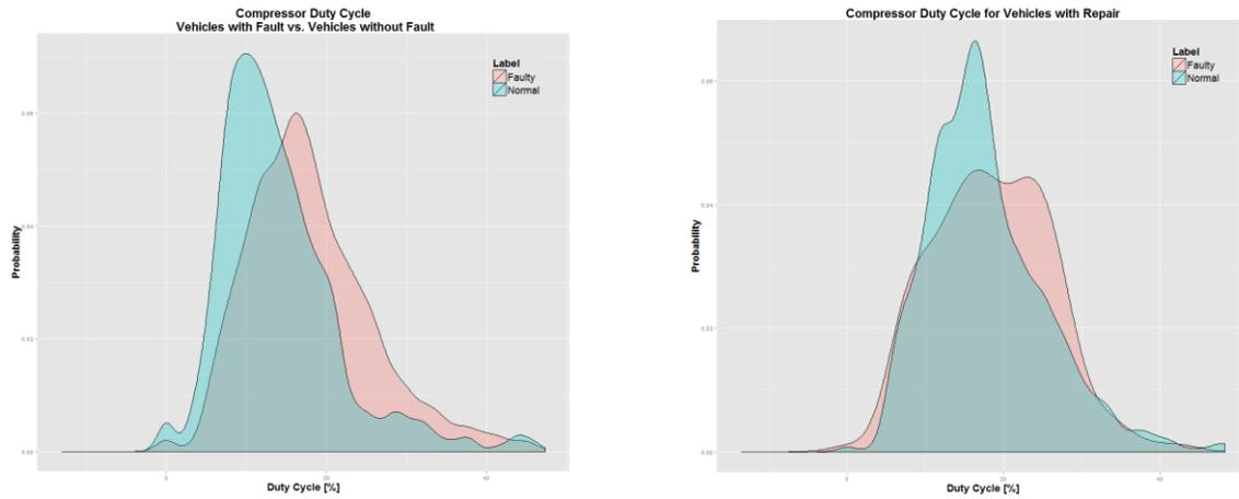
The second type of relation corresponds to different usage patterns, instead. Keeping with the same example, vehicles with compressor failures have a different distribution of “engine idle time” parameter than the ones without that fault (the red and blue plots, respectively, on the left figure below). However, there is no significant change between faulty vehicles long time before the fault (blue plot on the right figure) and the same vehicles short before the fault (red plot on the right).
