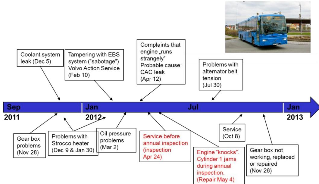
It turns out that there was a problem, probably lubrication, with one of the cylinders on this bus that eventually led to a jamming and required full engine renovation. Even despite customer complaints in April, the workshop was not aware of the issue and was not prepared for such a serious operation, which led to a significant delay (3 weeks) on top of an already lengthy repair. On the other hand, our method flagged the problem more than 20 weeks before it became a serious issue.
