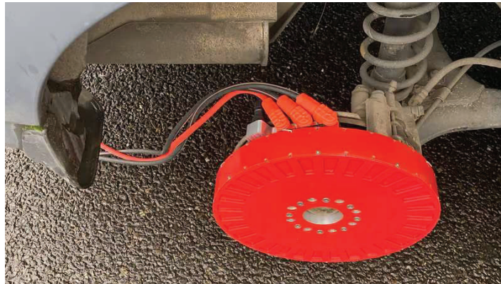
Fig. 20. REVR kit installed on car wheel
