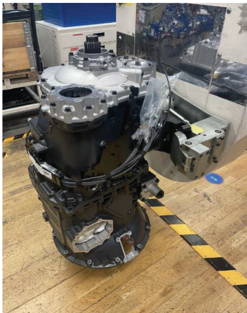
Figure 9: The gearbox after the assembly of the cable harness. (courtesy: Scania)
